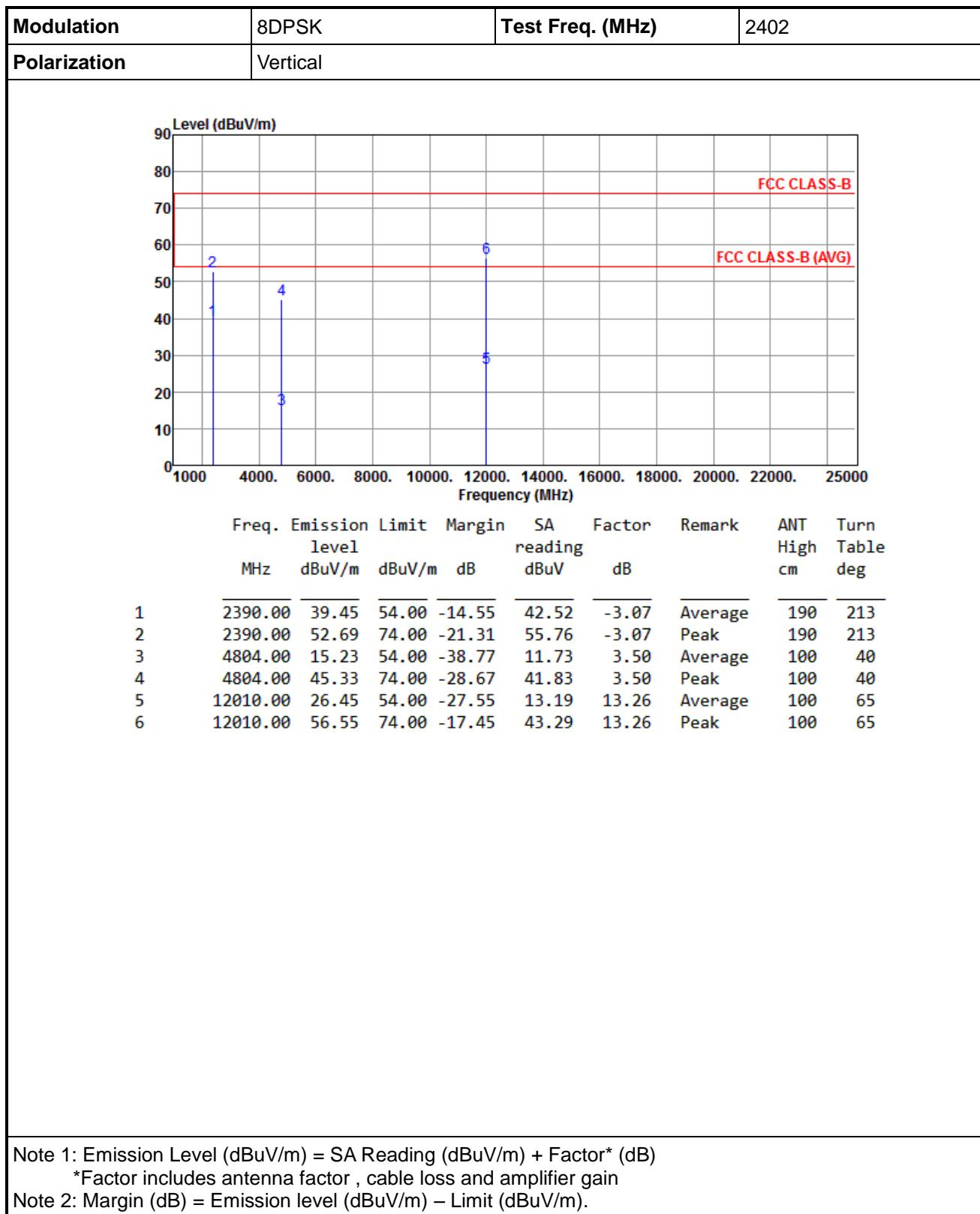
Note 1: Emission Level (dBuV/m) = SA Reading (dBuV/m) + Factor\* (dB)
