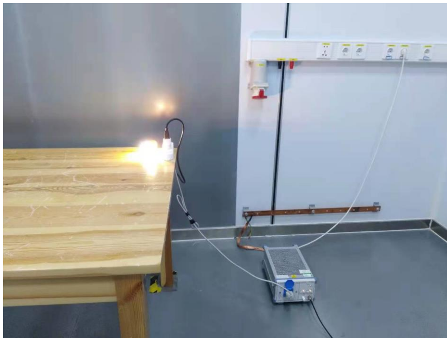
Fig. 4 Power line conducted emission setup photo
