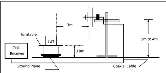
(c) For radiated emissions above 1000MHz
