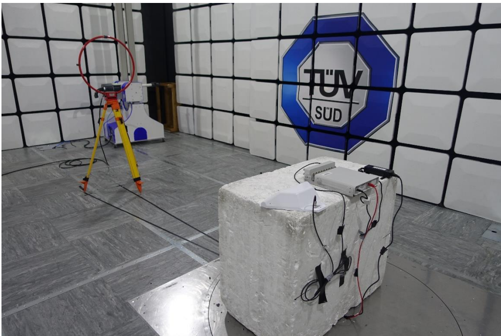
Figure 2 – Radiated Emissions Test Set Up
