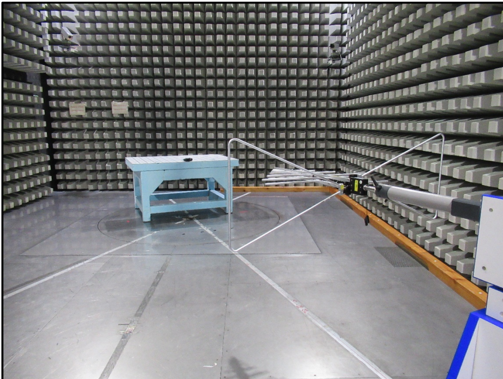
Photo 2: Radiated Test Setup-30 MHz to 1GHz
