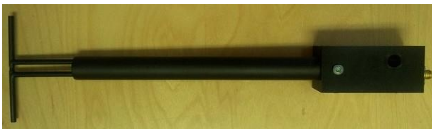
Figure 1 – MVG COMOSAR Validation Dipole
