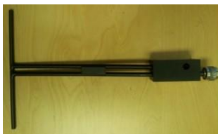
Figure 1 – MVG COMOSAR Validation Dipole
