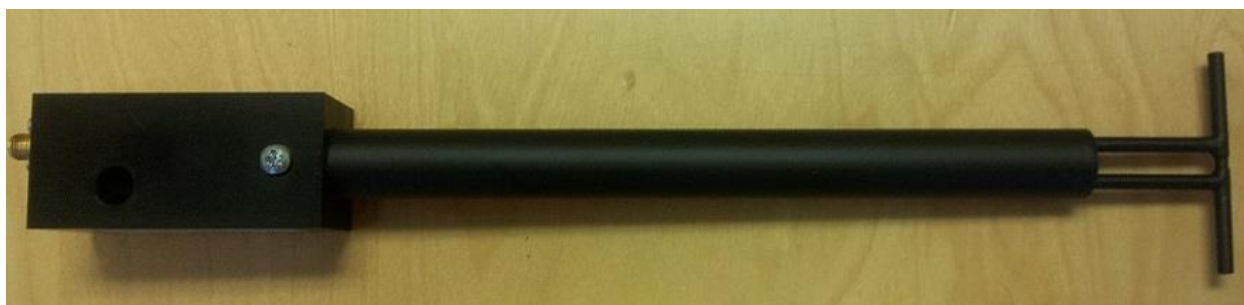
Figure 1 – MVG COMOSAR Validation Dipole
