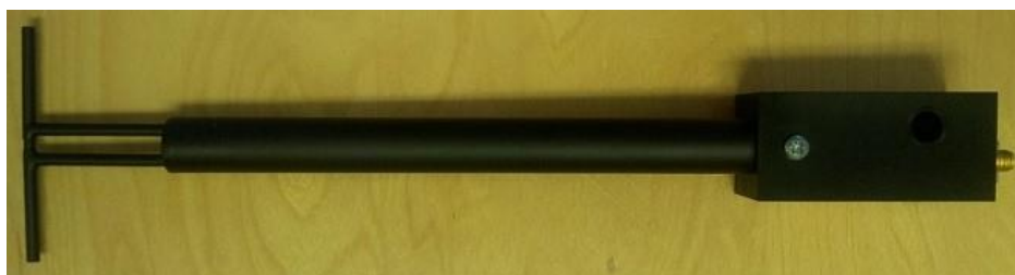
Figure 1 – MVG COMOSAR Validation Dipole
