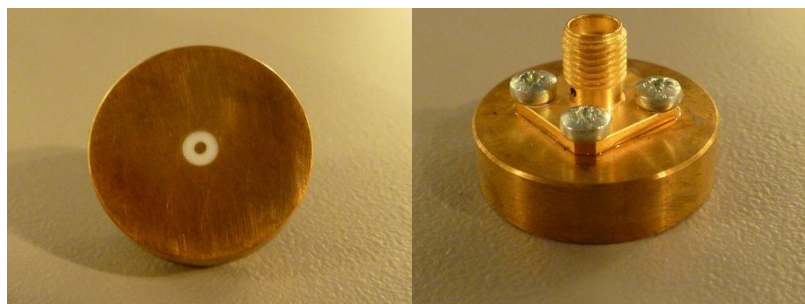
Figure 1 – MVG LIMESAR Dielectric Probe
