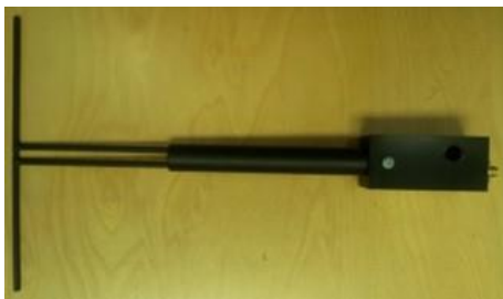
Figure 1 – MVG COMOSAR Validation Dipole
