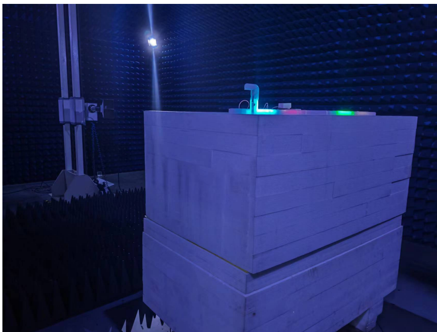
Photo of Radiated Emission Measurement (Above 1G)
