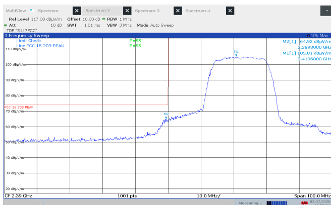
Lower Band Edge, 2412 MHz, 802.11g, 6Mb, Ant 1, Peak
