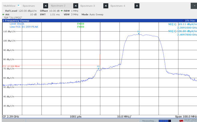
Lower Band Edge, 2412 MHz, 802.11g, 6Mb, Ant 2, Peak
