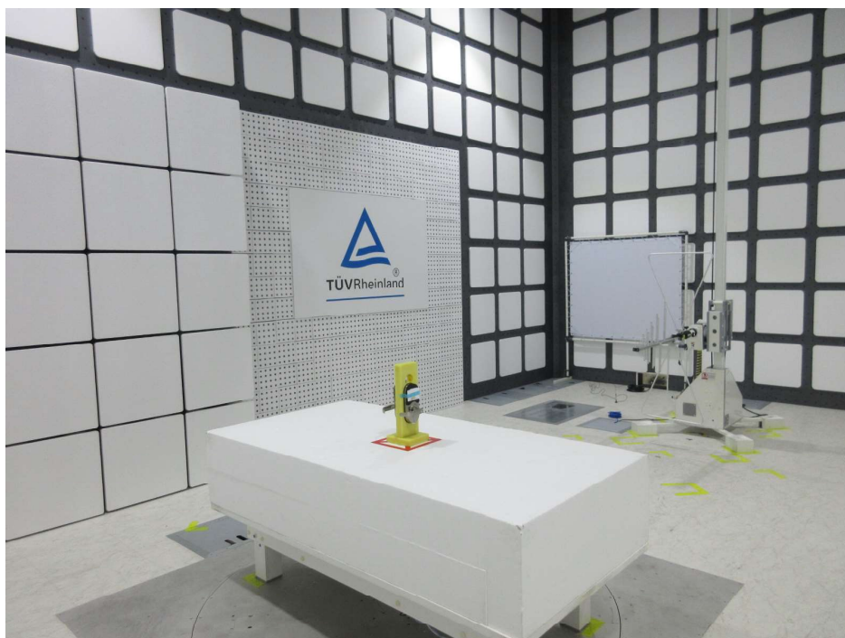
Photograph 2: Set-up for Spurious Emissions (Back View 1)
