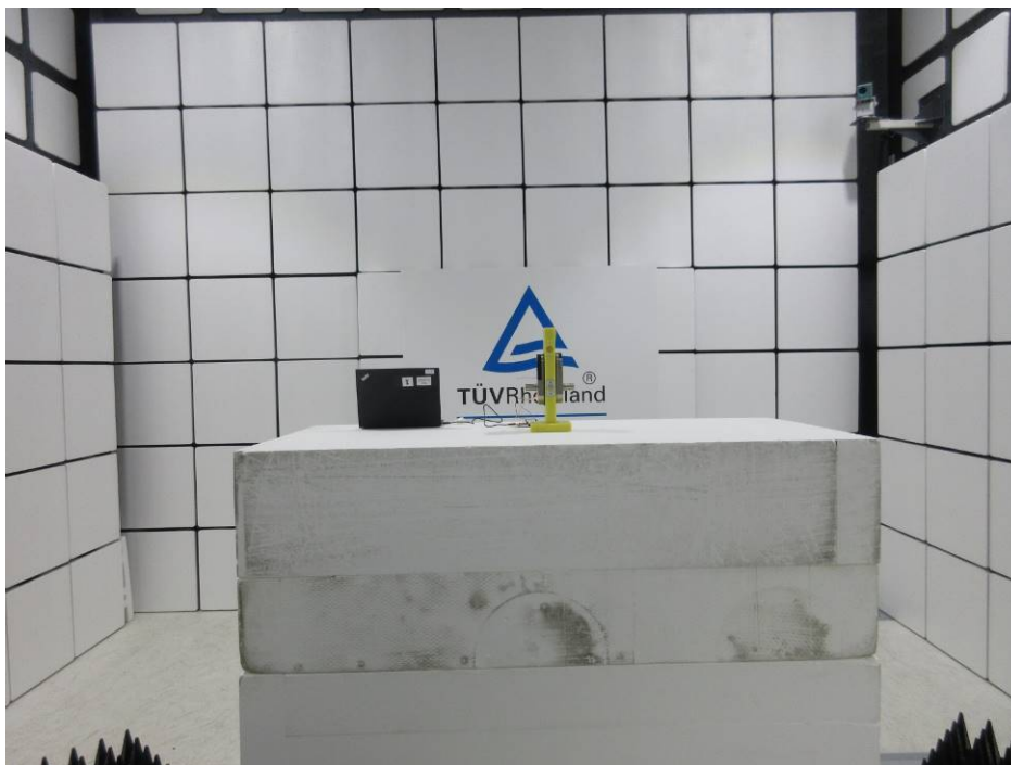
Photograph 2: Set-up for Spurious Emissions (Front View 2)
