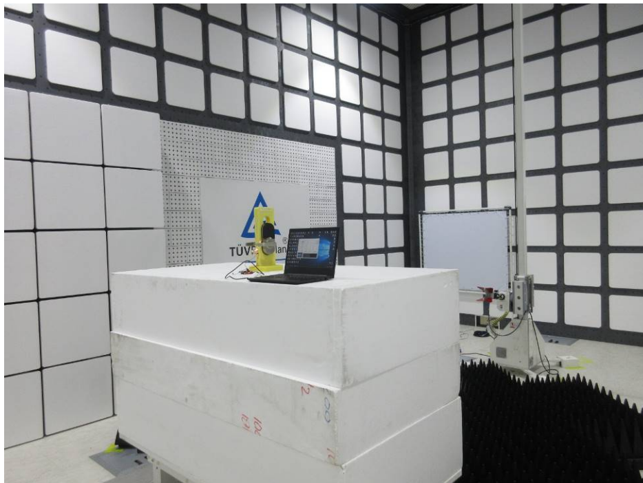
Photograph 4: Set-up for Spurious Emissions (Back View 2)
