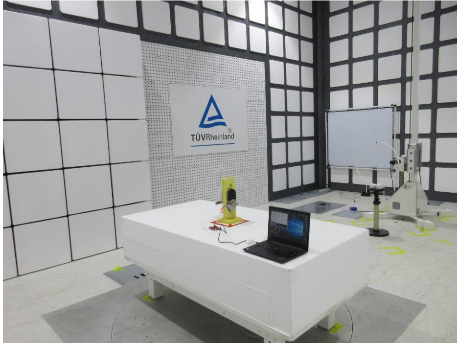
Photograph 5: Set-up for Spurious Emissions (Back View 3)
