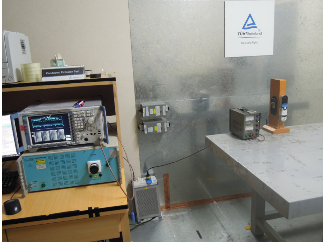
Photograph 6: Set-up for Main Emissions (Back View)
