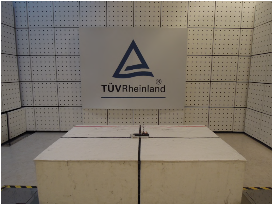
Photograph 2: Set-up for Spurious Emissions (Back View 1)
