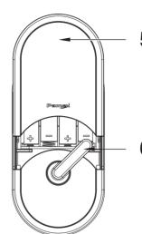
BATTERY COVER Protects the batteries from damage
