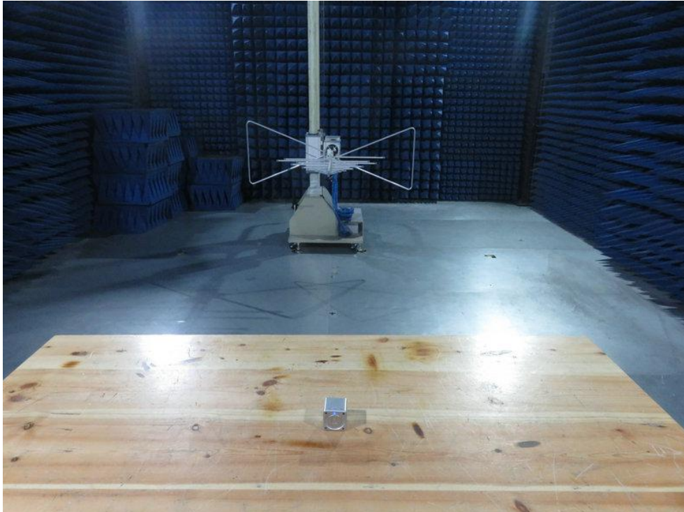
Photo of Radiation Emission Test
