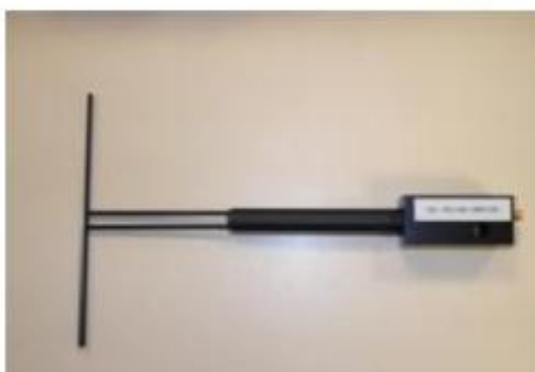
Figure 1 – Satimo COMOSAR Validation Dipole
