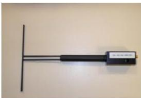
Figure 1 – Satimo COMOSAR Validation Dipole
