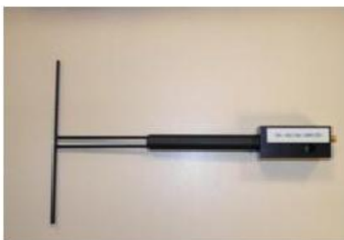
Figure 1 – Satimo COMOSAR Validation Dipole
