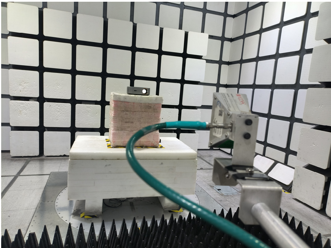
Radiated Emissions View (18-25 GHz)
