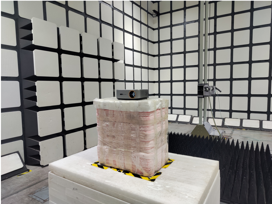
Radiated Emissions View (18-25 GHz)
