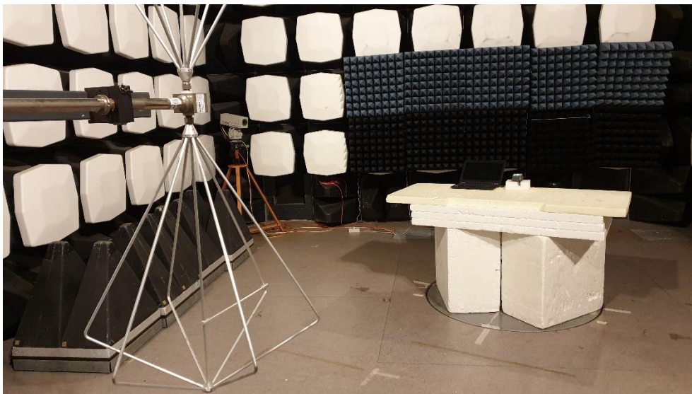
Photo 3. Radiated emission test setup for 30 - 200 MHz.
