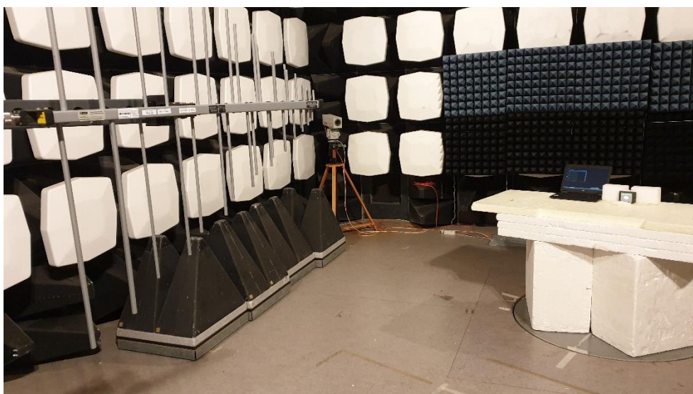
Photo 4. Radiated emission test setup for 200 - 1000 MHz.
