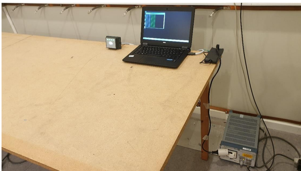
Photo 6 - Conducted emission test setup.
