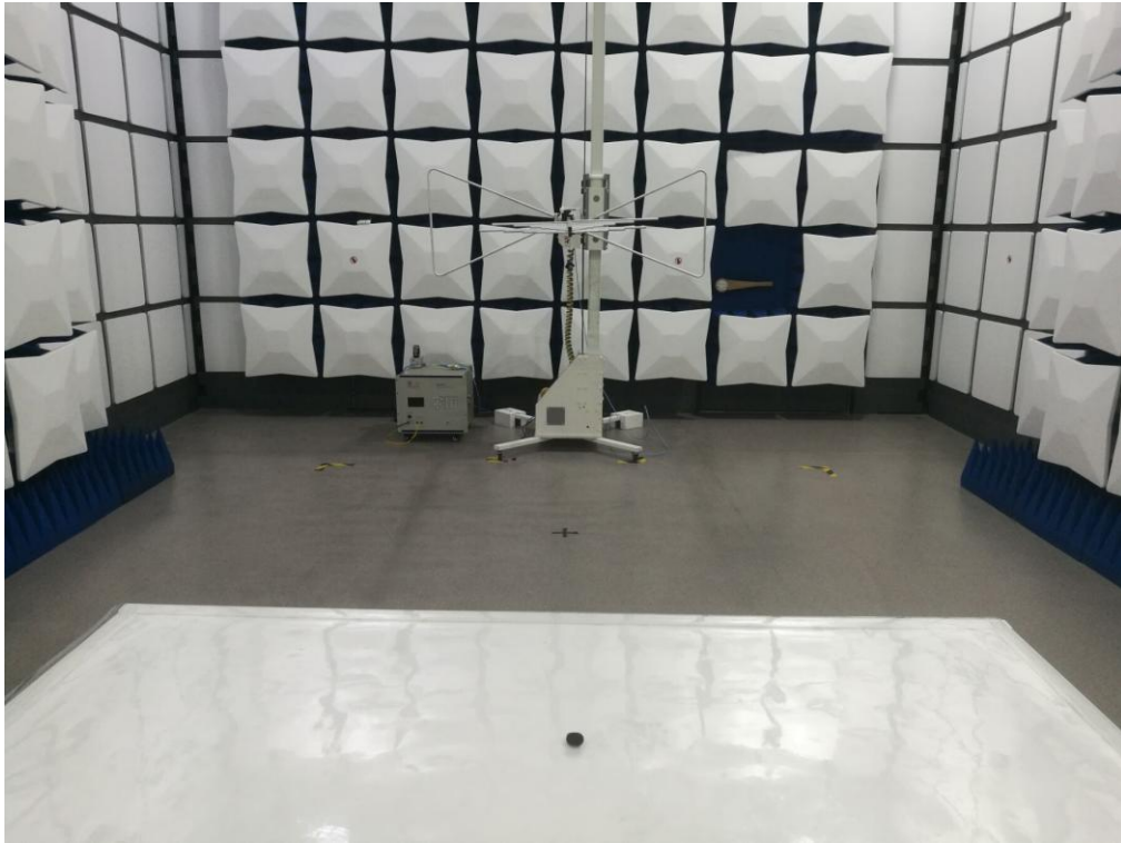
FCC RADIATED EMISSION TEST SETUP
