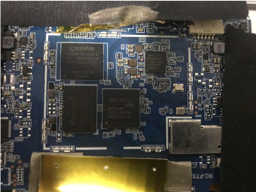
Mainboard Model No.: RS512M32LM4D2BDS-53BT 2GB & EMMC32G-TA28 32GB
