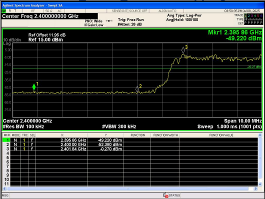
Out Of Band Emission(Left) 8DPSK_3-DH5_Channel Hopping
