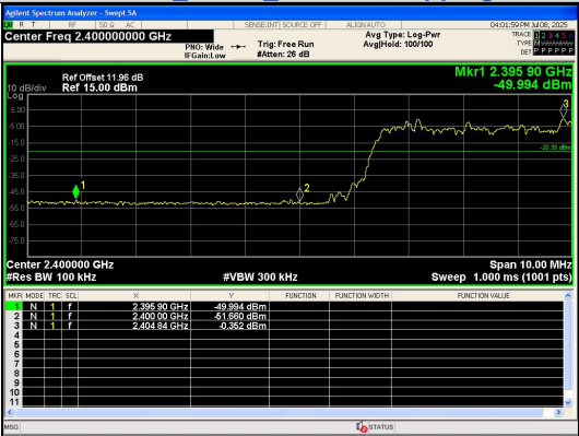
Out Of Band Emission(Left) 8DPSK_3-DH5_Channel Hopping
