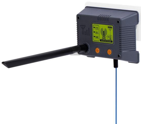
(Note: The receiving antenna can extend downward directly or can be attached to the curtain from above.)
