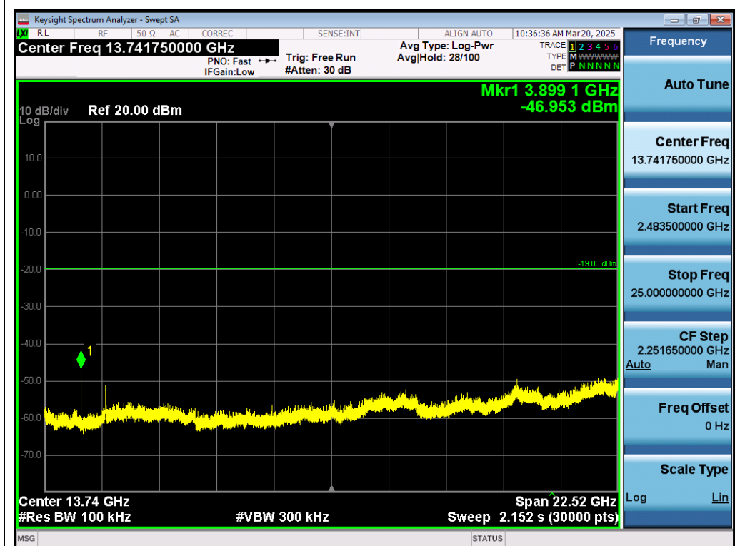
Test_Graph_802.11ax20_ANT1_2437_MCS0_Higher Band Emissions
