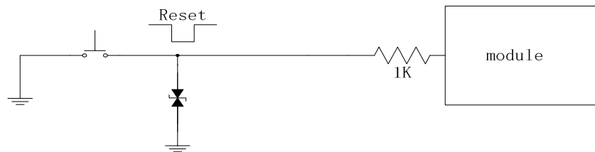
Figure 4.7: Reference design of key reset circuit
