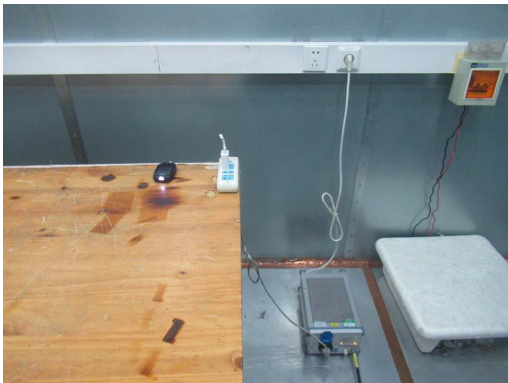
Picture 2: Conducted Emissions Test Setup
