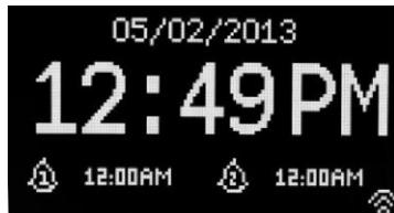
A **splash screen** is displayed for each mode. Press source to cycle through the listening modes.
