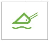
1) This lamp lights ON when the boom float is activated.
