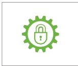
① This lamp lights ON when the torque converter lock up function is operating.
