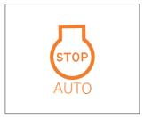
① This lamp lights ON when the engine auto shutdown function is activated.
