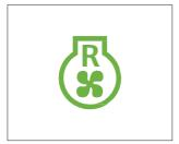
① This lamp lights ON when the cooling fan reverse mode is acti-vated
