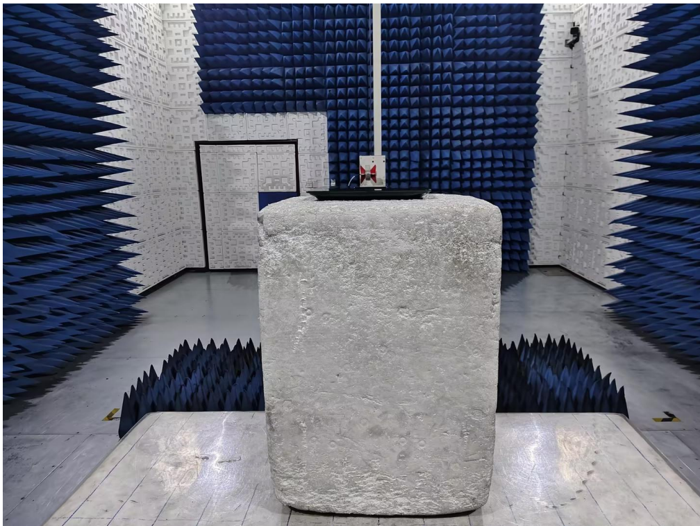
RADIATED EMISSION TEST SETUP ABOVE 1GHz
