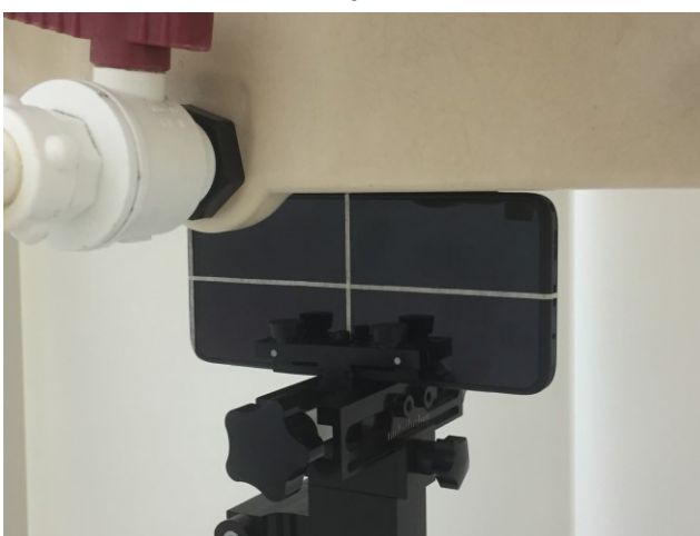
Right Side, Test Separation 0 mm
