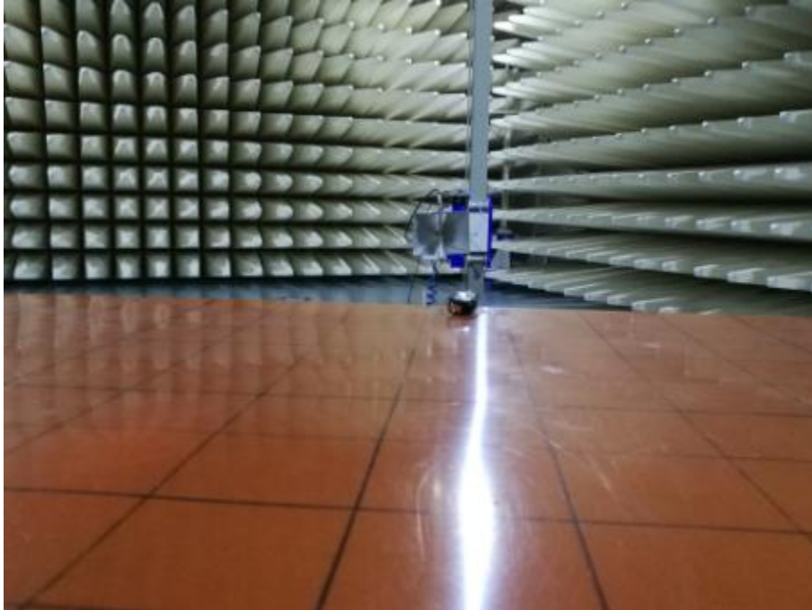
Radiated Emissions Test Setup: 1000MHz-6000MHz
