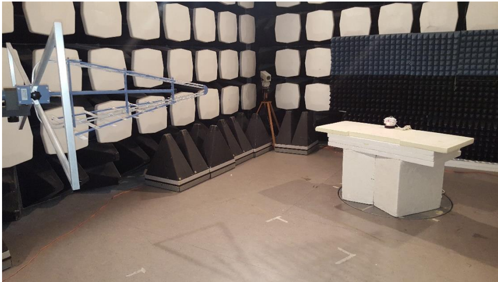
Photo 3 - Radiated emission test setup for 30 - 1000 MHz.
