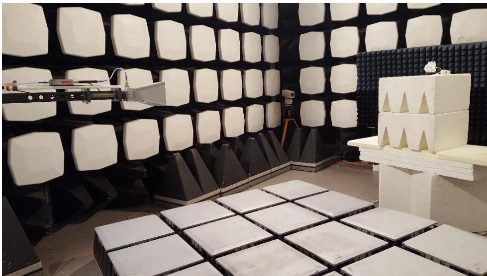
Photo 4 - Radiated emission test setup for 1 - 14 GHz.
