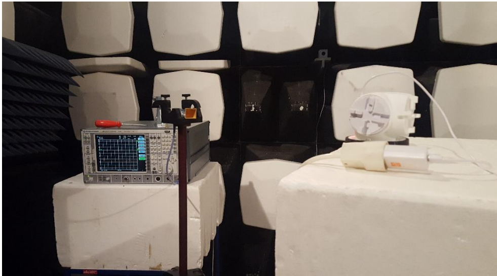
Photo 5. Radiated emission test setup for 14 – 25 GHz.
