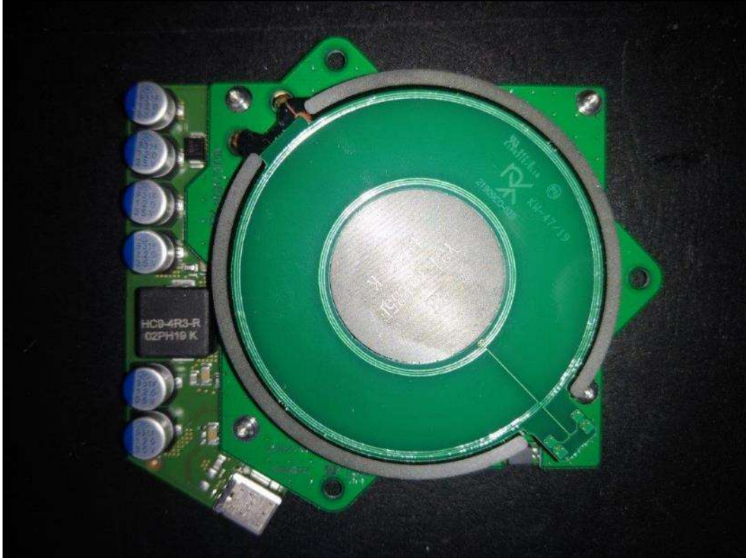
Photo 1: DUT - Receiver 81909002 (60W)
