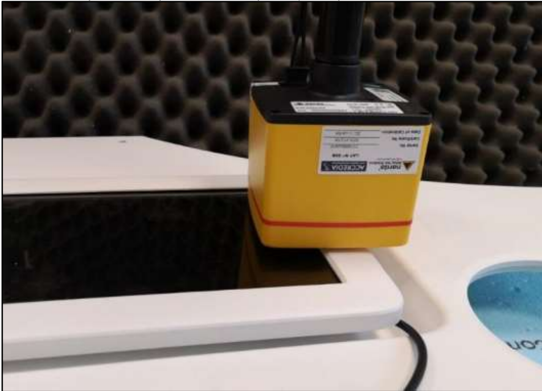
Photo 16: Test position - side with EHP 50F probe (touch position and worst case orientation)
