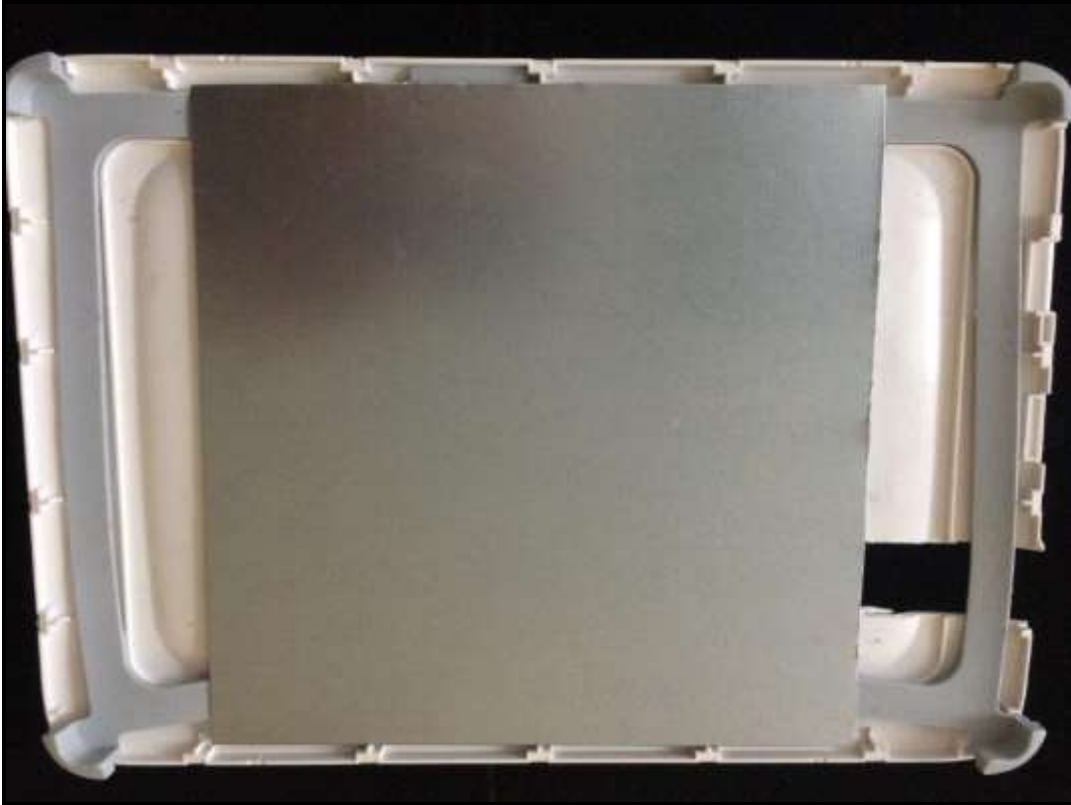
Photo 21: Test position – Top side with EHP 50F probe - Receiver with shield metal (no tablet)
