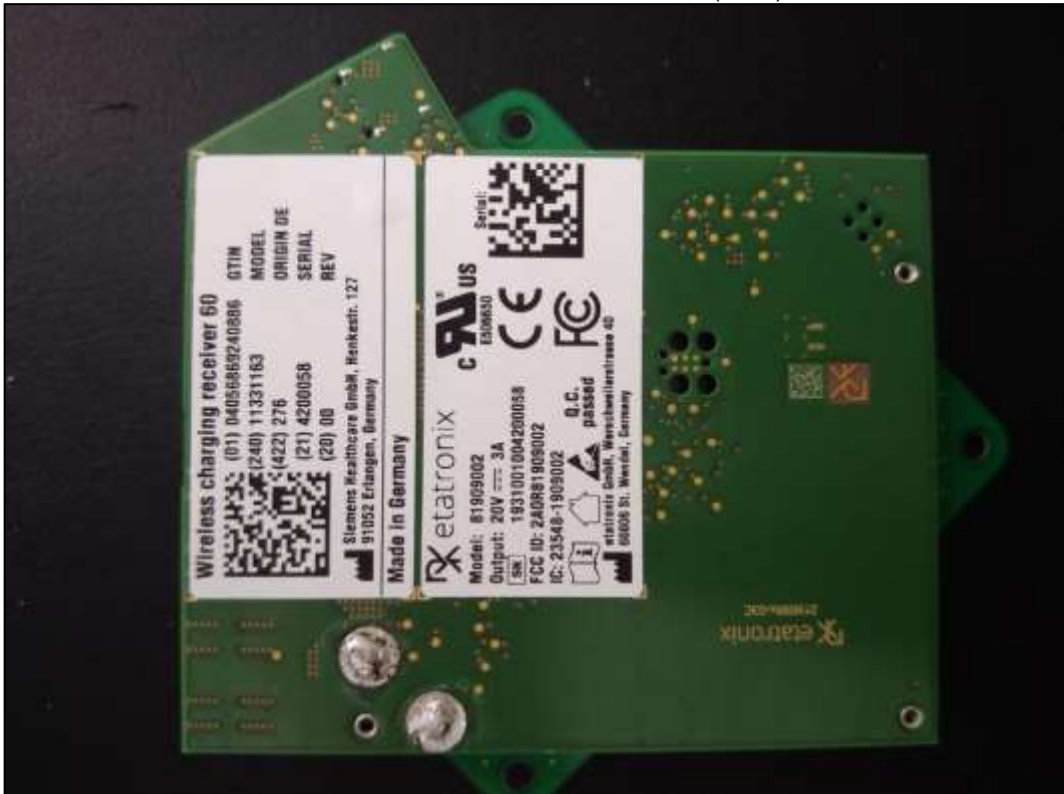
Photo 2: DUT - Receiver 81909002 (60W)
