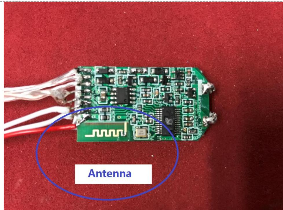
Details of: Internal PCB bottom view
