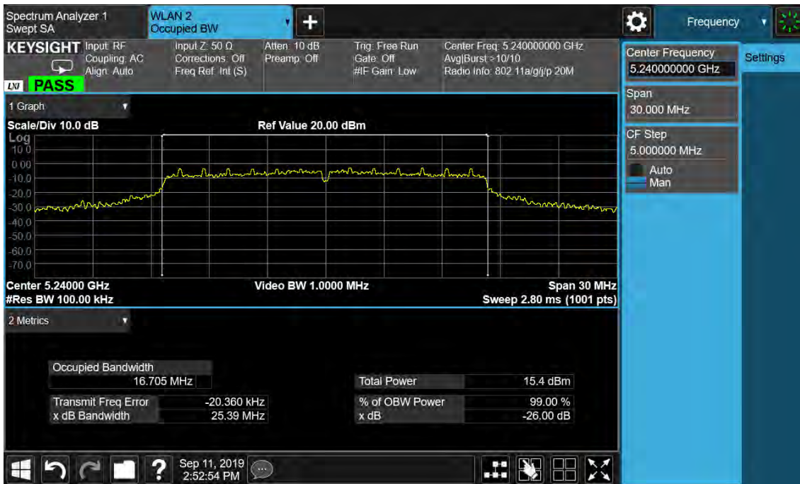
Figure 3: 26dB Bandwidth and 99% Bandwidth, 802.11a, 5240MHz
