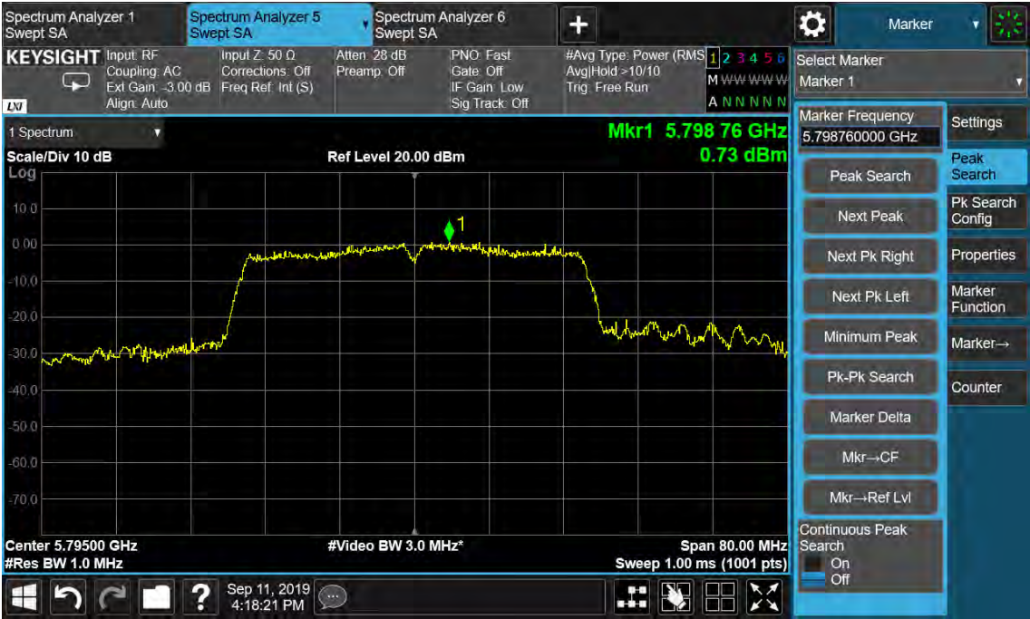
Figure 69: Power Spectral Density, 802.11ac(VHT40), 5785MHz
