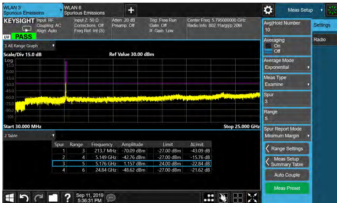
Figure 71: Undesirable Emission, 30MHz-25GHz, 802.11a, 5180MHz
