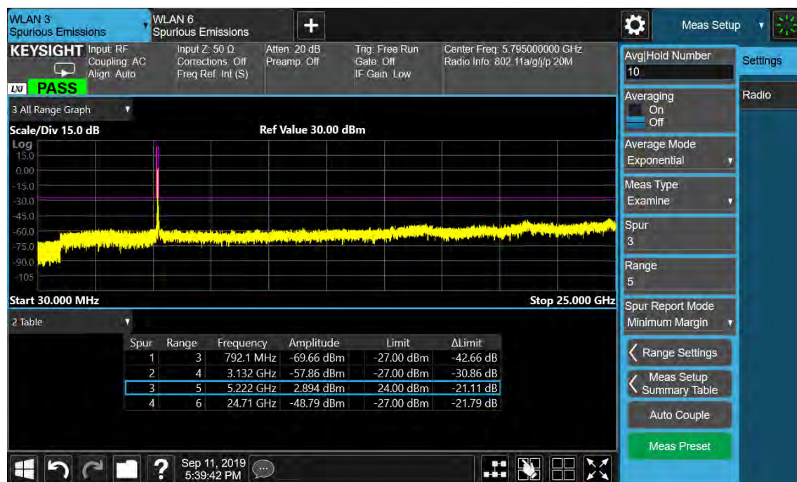
Figure 78: Undesirable Emission, 30MHz-25GHz, 802.11ac(VHT20), 5220MHz
