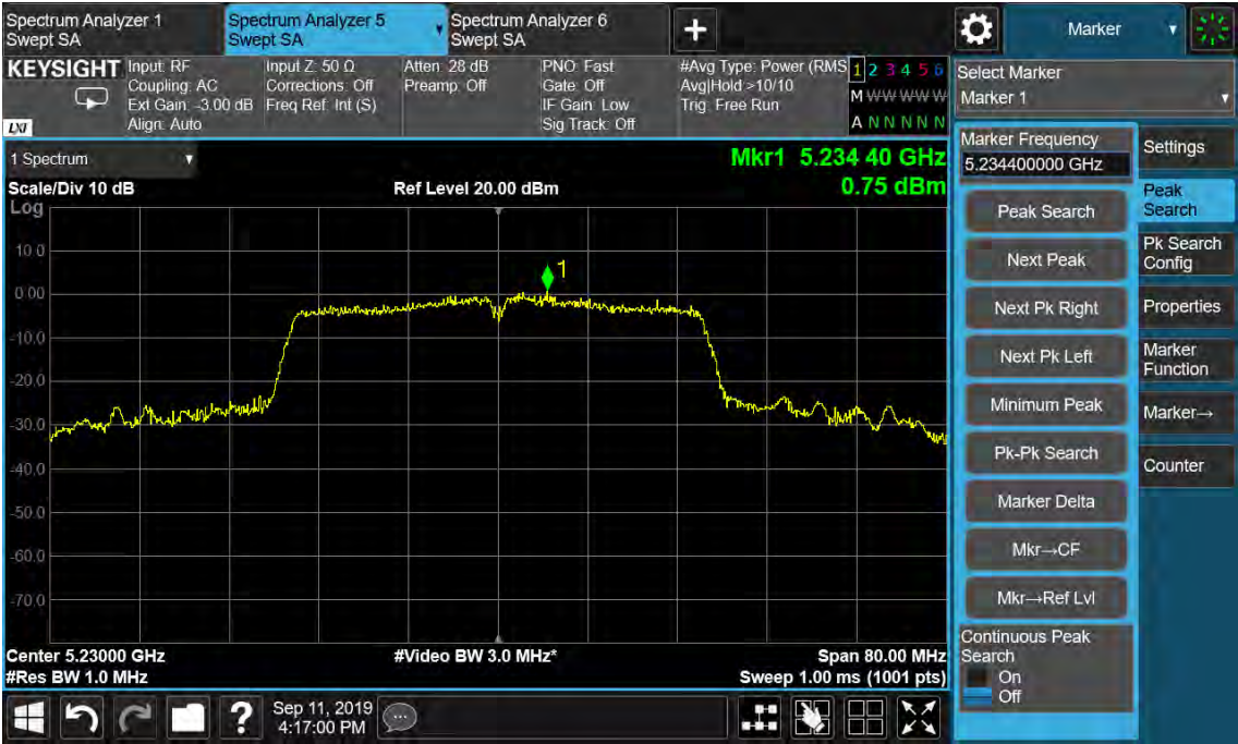
Figure 55: Power Spectral Density, 802.11ac(VHT40), 5230MHz
