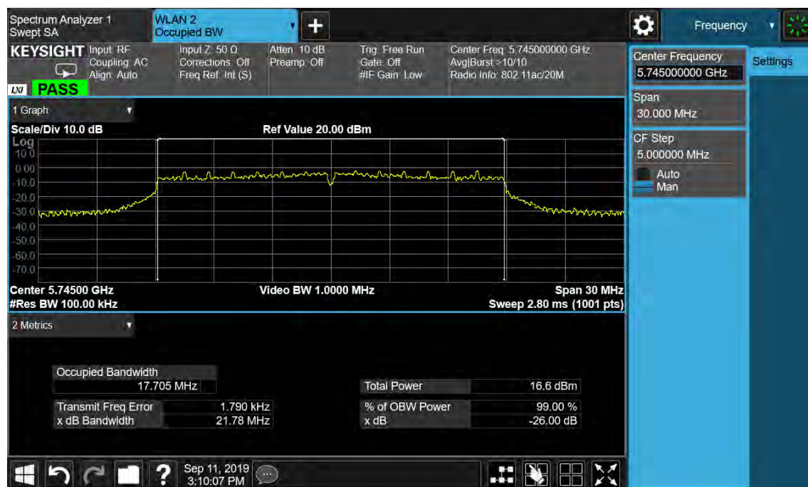
Figure 21: 26dB Bandwidth and 99% Bandwidth, 802.11ac(VHT20), 5745MHz
