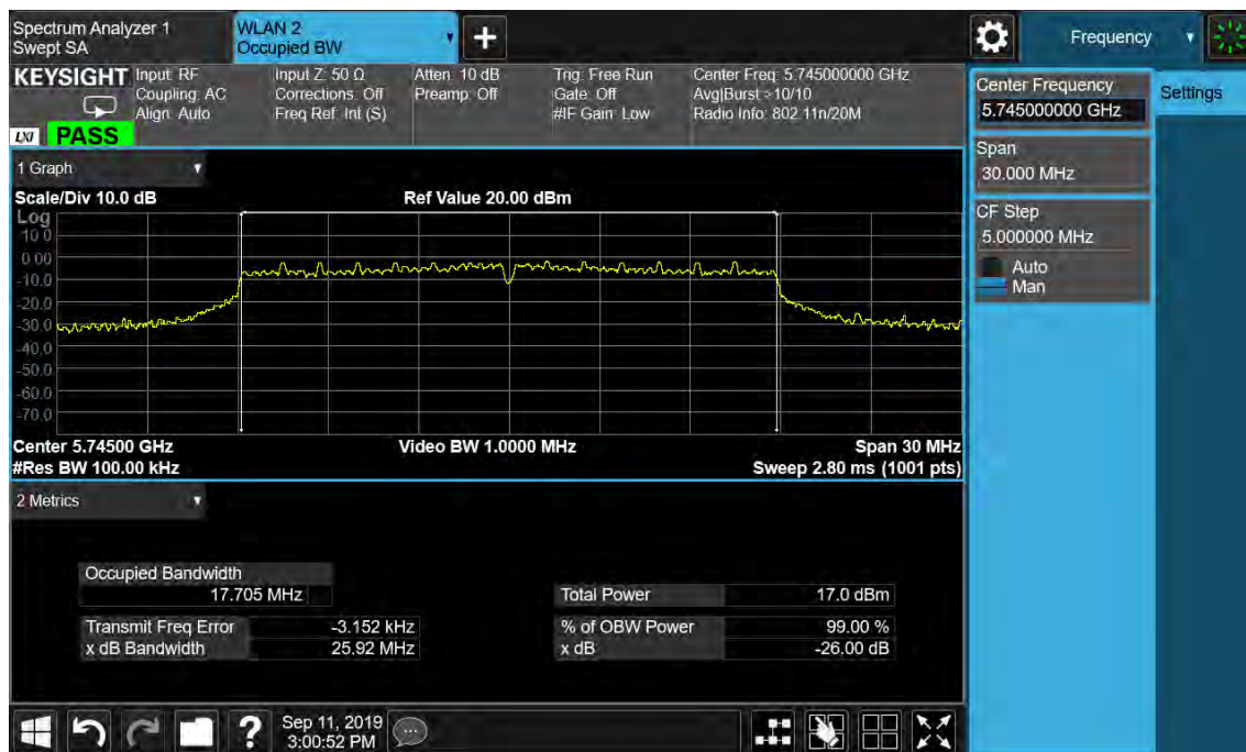
Figure 18: 26dB Bandwidth and 99% Bandwidth, 802.11n(HT20), 5745MHz
