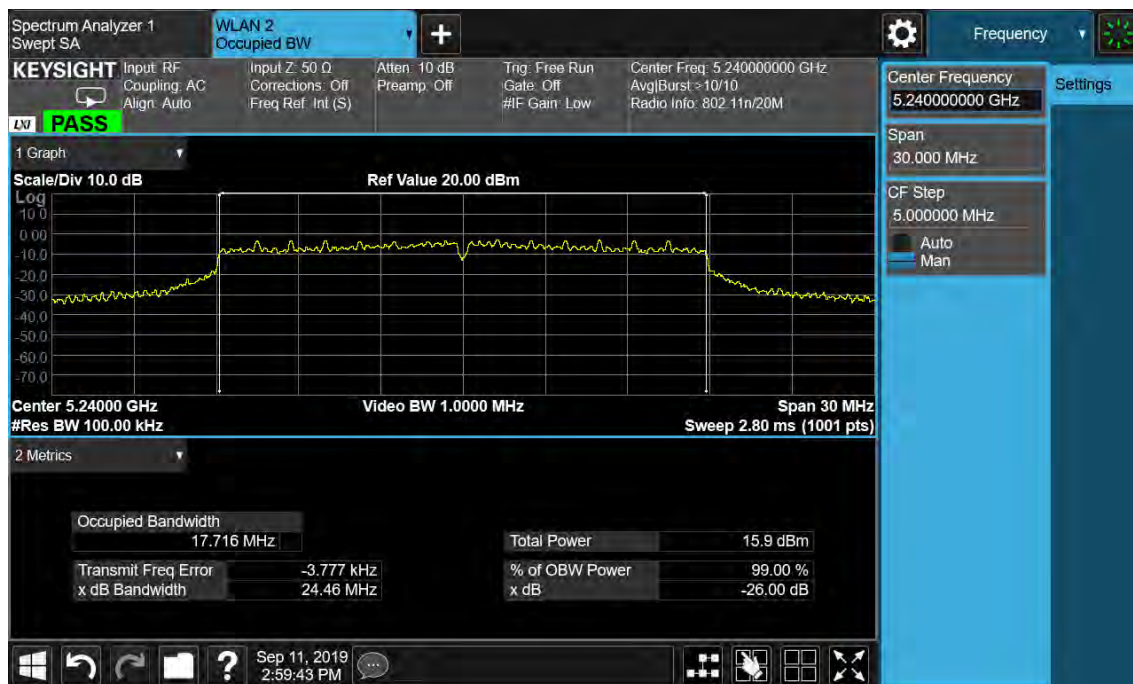
Figure 6: 26dB Bandwidth and 99% Bandwidth, 802.11n(HT20), 5240MHz
