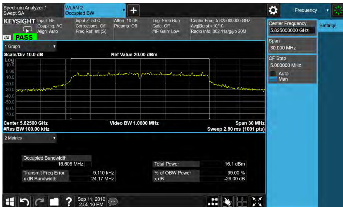
Figure 17: 26dB Bandwidth and 99% Bandwidth, 802.11a, 5825MHz
