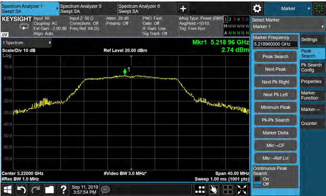
Figure 44: Power Spectral Density, 802.11a, 5220MHz
