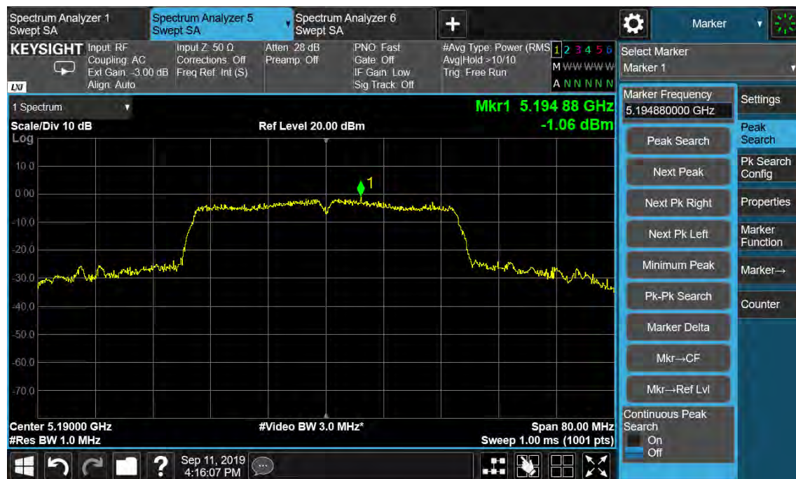
Figure 54: Power Spectral Density, 802.11ac(VHT40), 5190MHz
