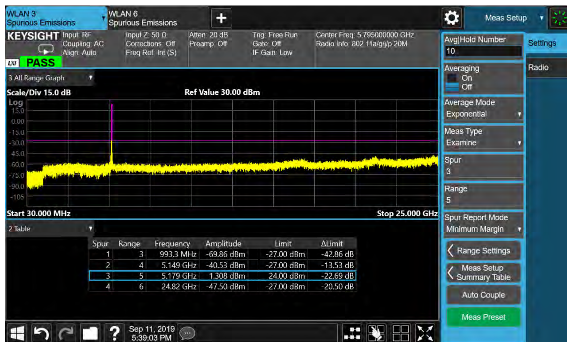
Figure 77: Undesirable Emission, 30MHz-25GHz, 802.11ac(VHT20), 5180MHz
