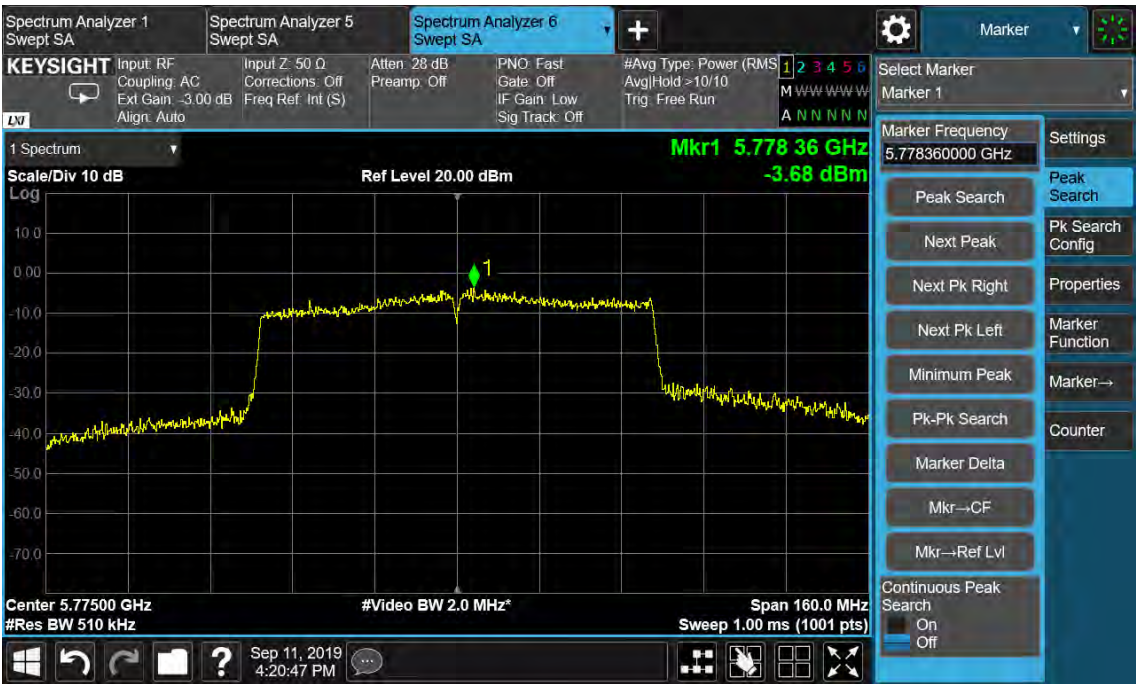
Figure 70: Power Spectral Density, 802.11ac(VHT80), 5775MHz
