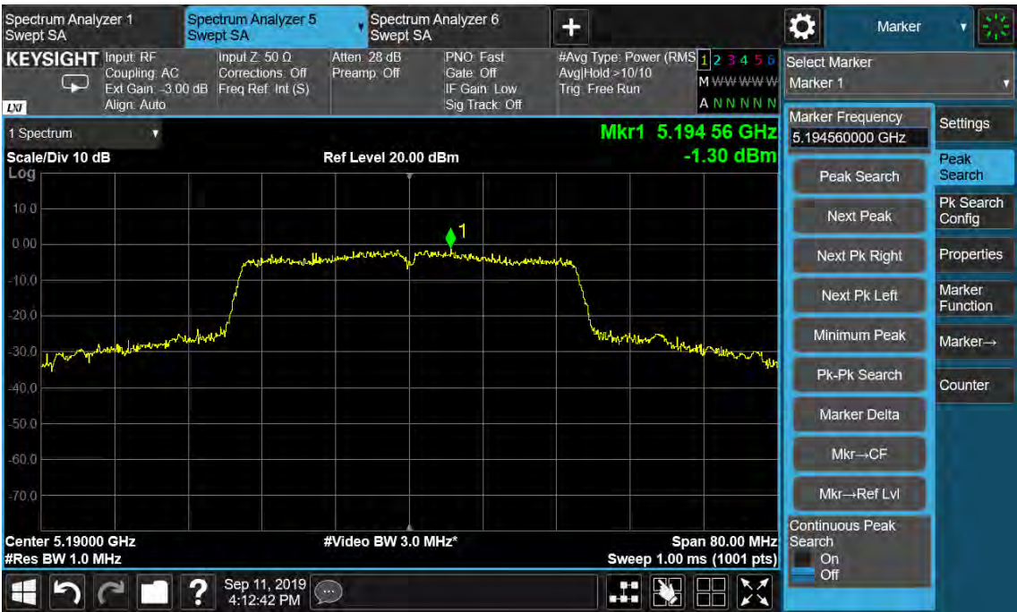
Figure 52: Power Spectral Density, 802.11n(HT40), 5190MHz
