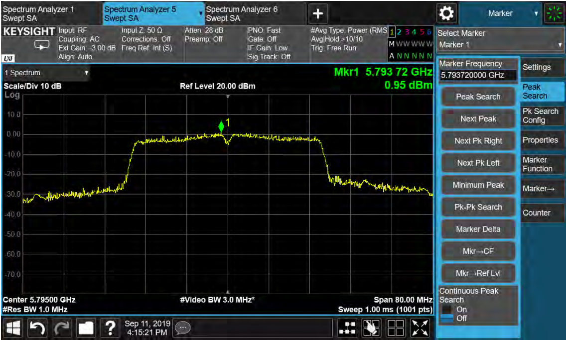
Figure 67: Power Spectral Density, 802.11n(HT40), 5795MHz
