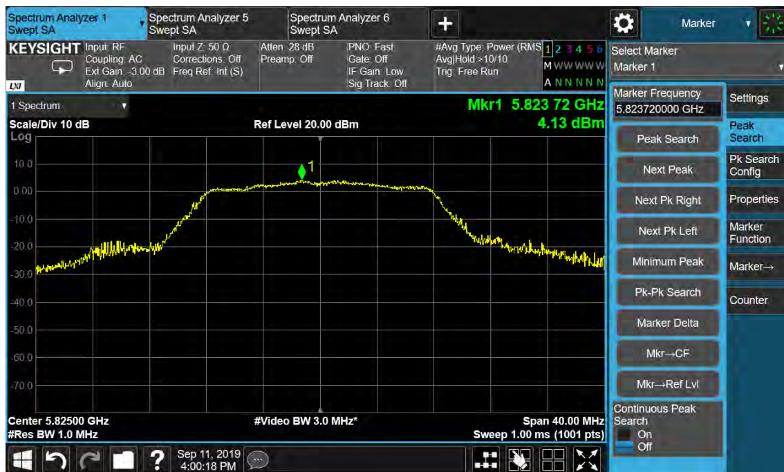
Figure 59: Power Spectral Density, 802.11a, 5825MHz
