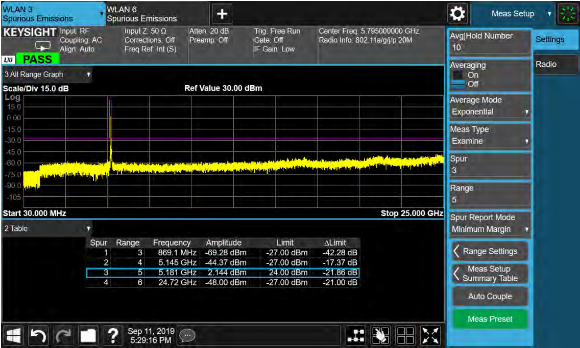
Figure 73: Undesirable Emission, 30MHz-25GHz, 802.11a, 5240MHz
