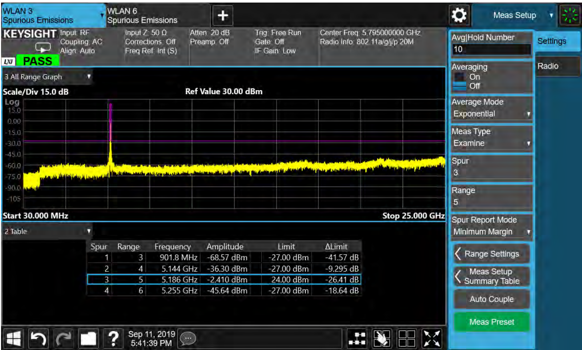
Figure 82: Undesirable Emission, 30MHz-25GHz, 802.11ac(VHT40), 5190MHz
