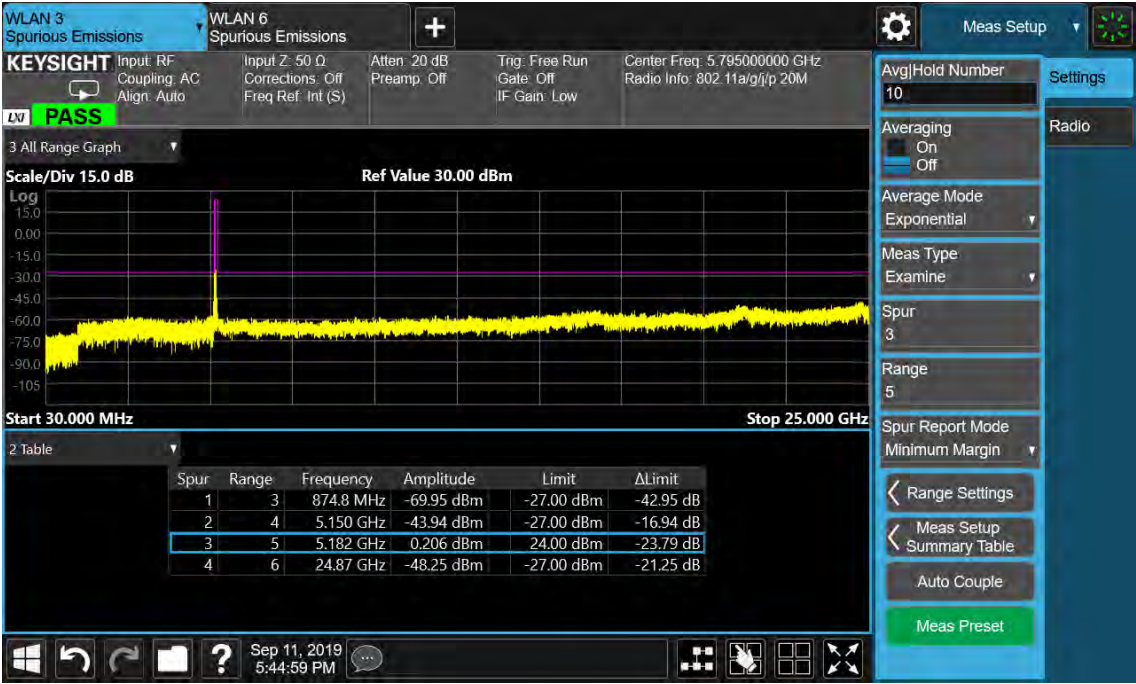
Figure 74: Undesirable Emission, 30MHz-25GHz, 802.11n(HT20), 5180MHz
