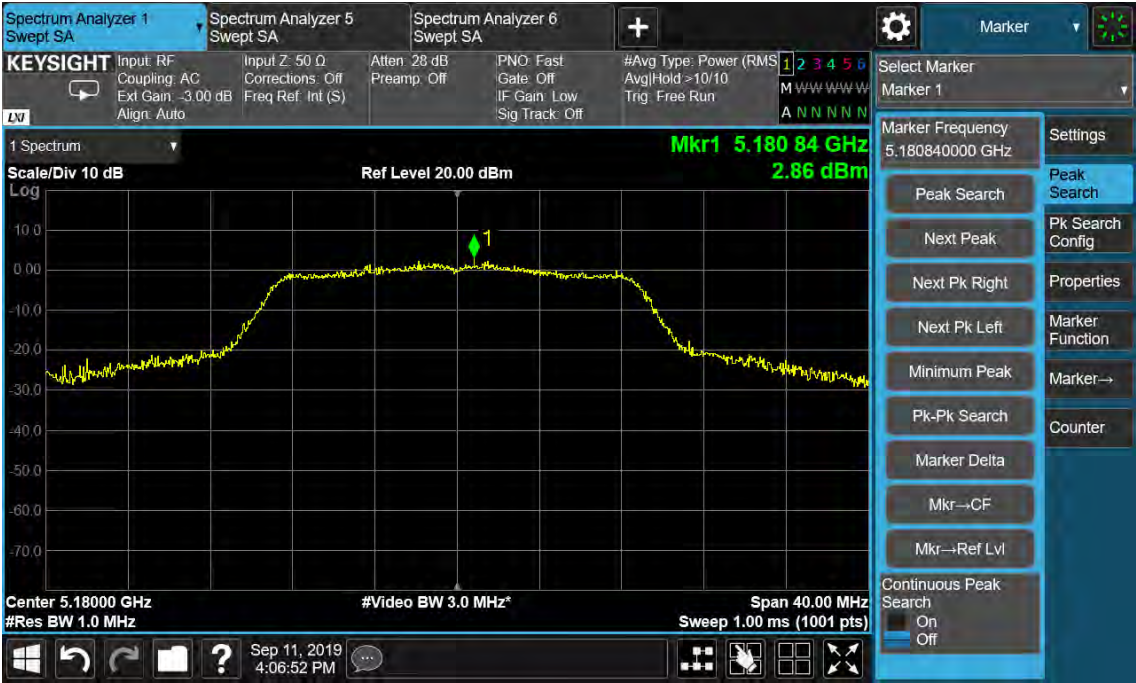
Figure 49: Power Spectral Density, 802.11ac(VHT20), 5180MHz
