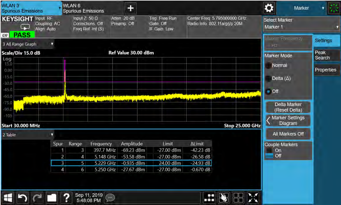
Figure 81: Undesirable Emission, 30MHz-25GHz, 802.11n(HT40), 5230MHz
