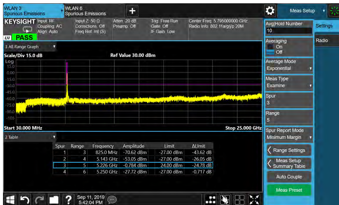
Figure 83: Undesirable Emission, 30MHz-25GHz, 802.11ac(VHT40), 5230MHz
