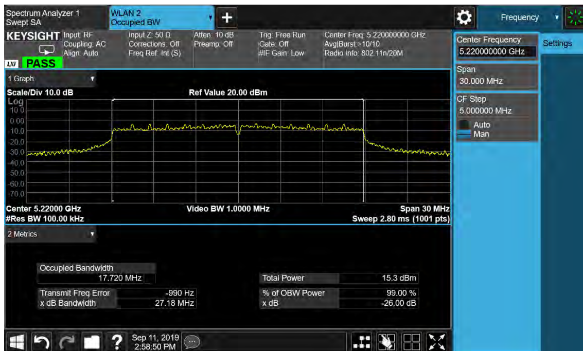
Figure 5: 26dB Bandwidth and 99% Bandwidth, 802.11n(HT20), 5220MHz
