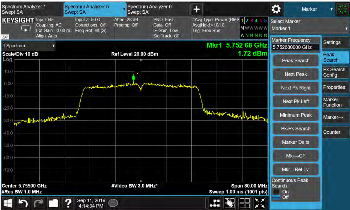
Figure 66: Power Spectral Density, 802.11n(HT40), 5755MHz
