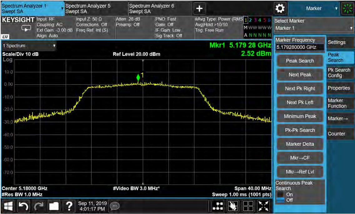
Figure 46: Power Spectral Density, 802.11n(HT20), 5180MHz
