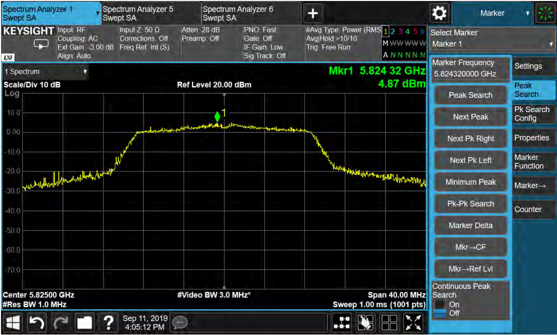
Figure 62: Power Spectral Density, 802.11n(HT20), 5825MHz
