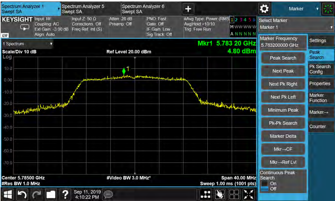
Figure 64: Power Spectral Density, 802.11ac(VHT20), 5785MHz
