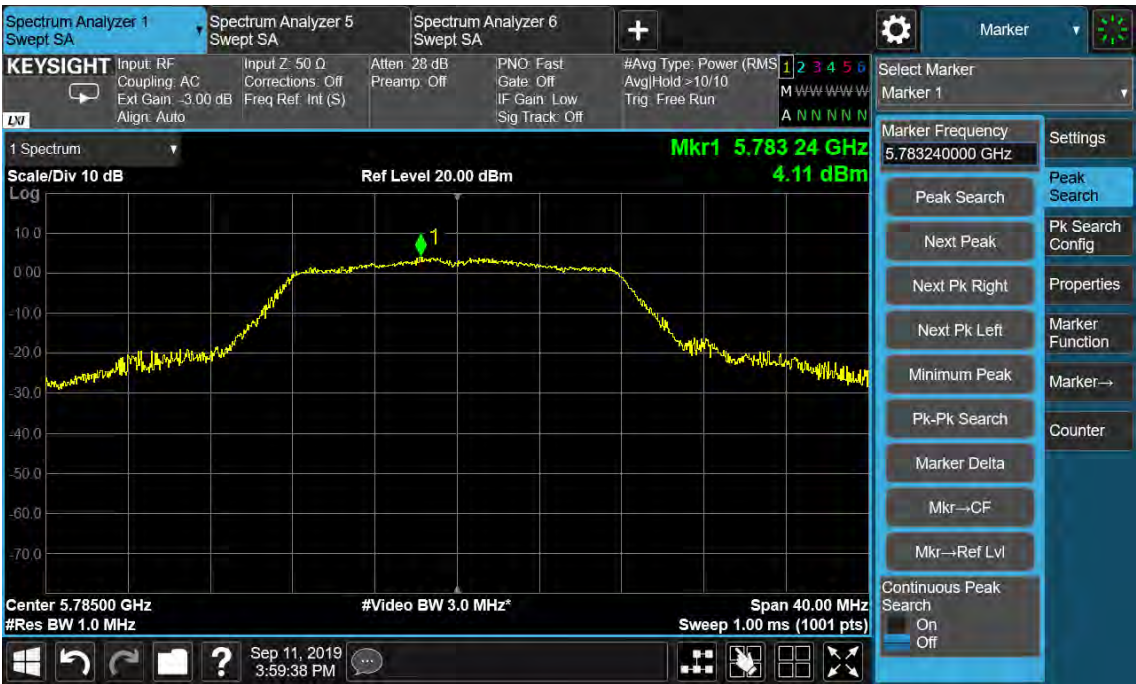
Figure 58: Power Spectral Density, 802.11a, 5785MHz
