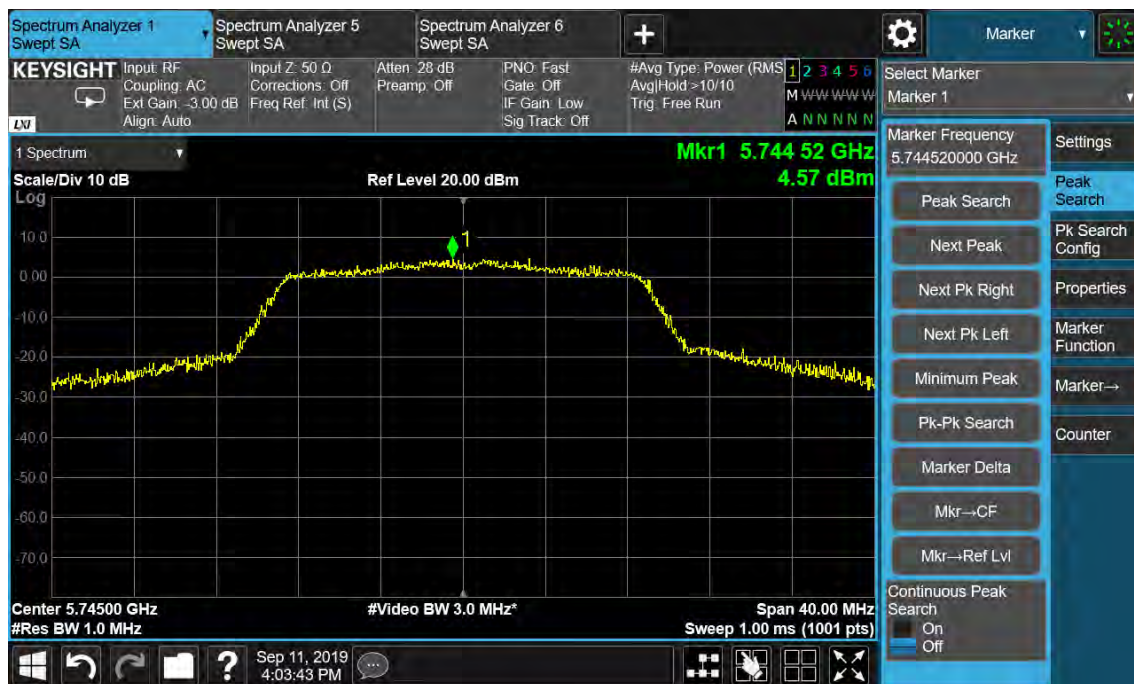
Figure 60: Power Spectral Density, 802.11n(HT20), 5745MHz
