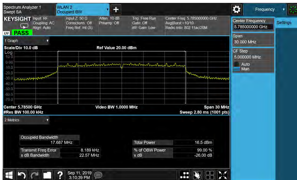
Figure 22: 26dB Bandwidth and 99% Bandwidth, 802.11ac(VHT20), 5785MHz
