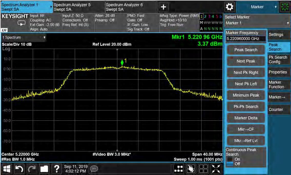
Figure 47: Power Spectral Density, 802.11n(HT20), 5220MHz
