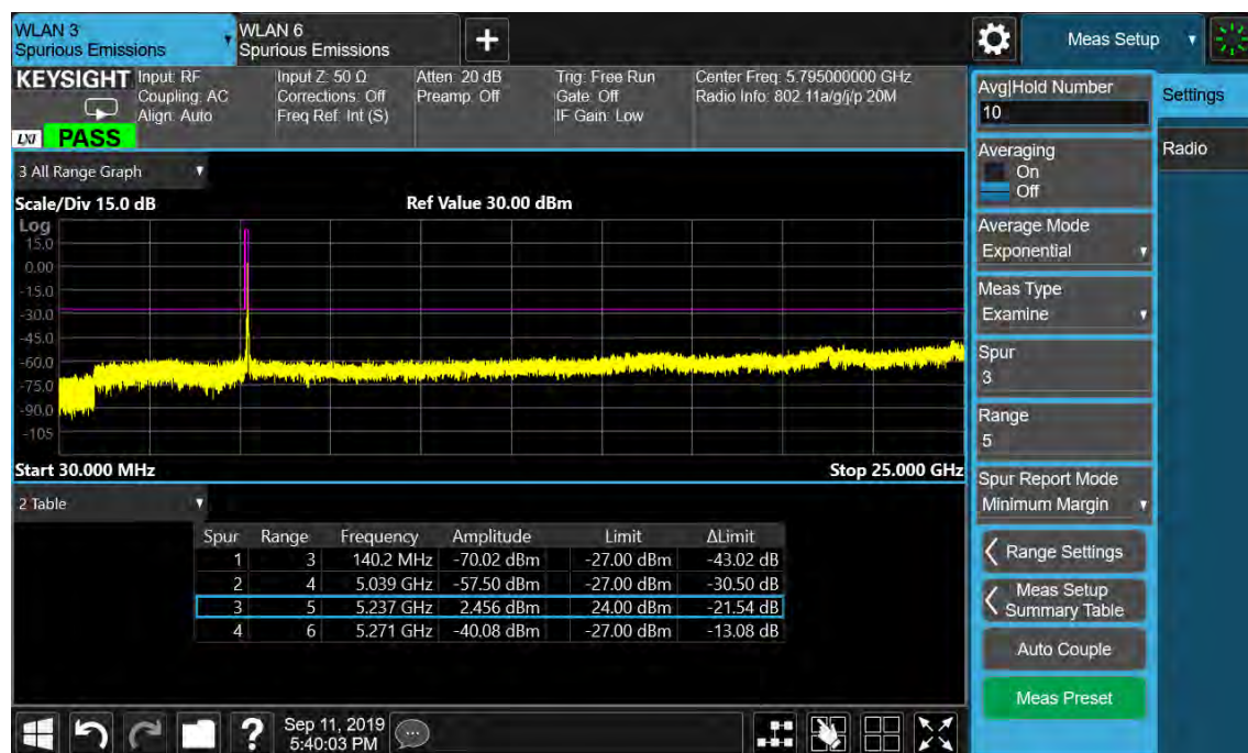
Figure 79: Undesirable Emission, 30MHz-25GHz, 802.11ac(VHT20), 5240MHz
