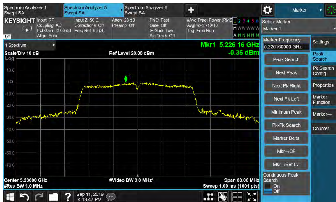
Figure 53: Power Spectral Density, 802.11n(HT40), 5230MHz
