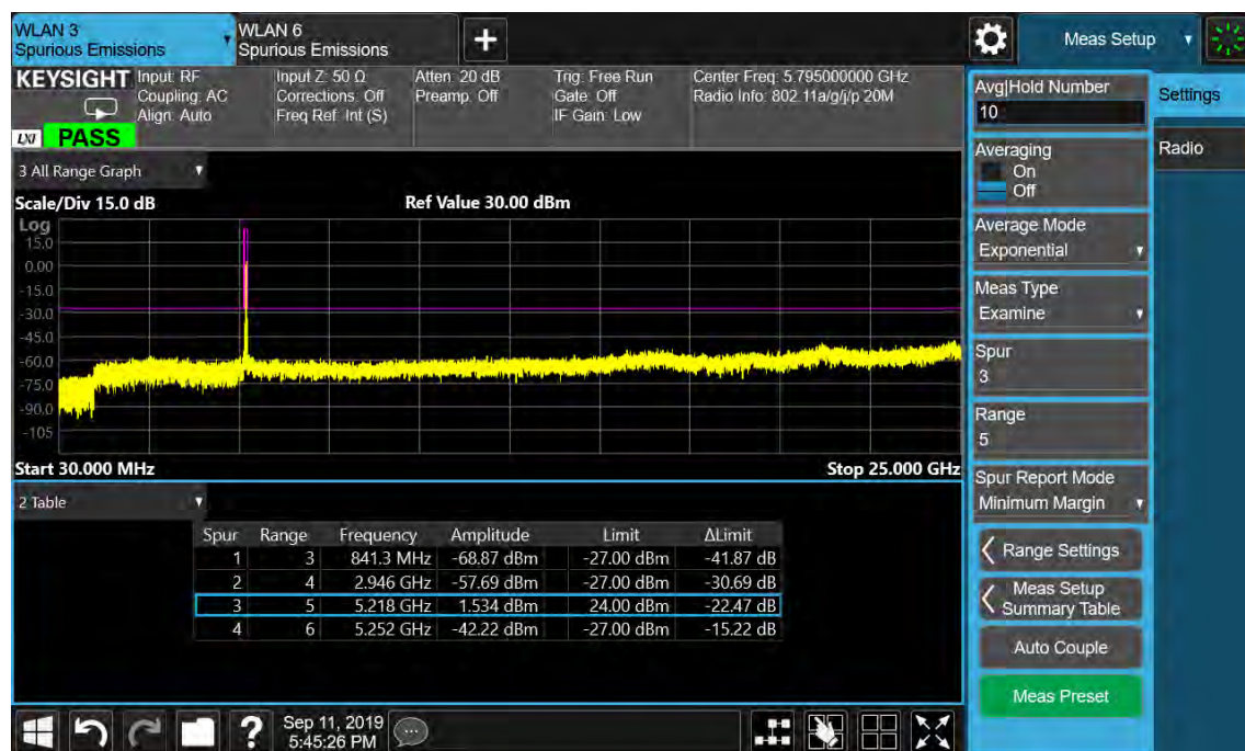
Figure 75: Undesirable Emission, 30MHz-25GHz, 802.11n(HT20), 5220MHz
