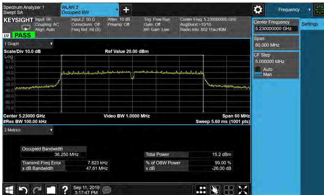
Figure 13: 26dB Bandwidth and 99% Bandwidth, 802.11ac(VHT40), 5230MHz
