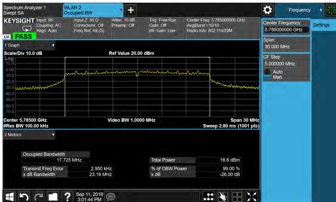
Figure 19: 26dB Bandwidth and 99% Bandwidth, 802.11n(HT20), 5785MHz
