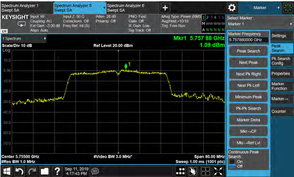
Figure 68: Power Spectral Density, 802.11ac(VHT40), 5755MHz
