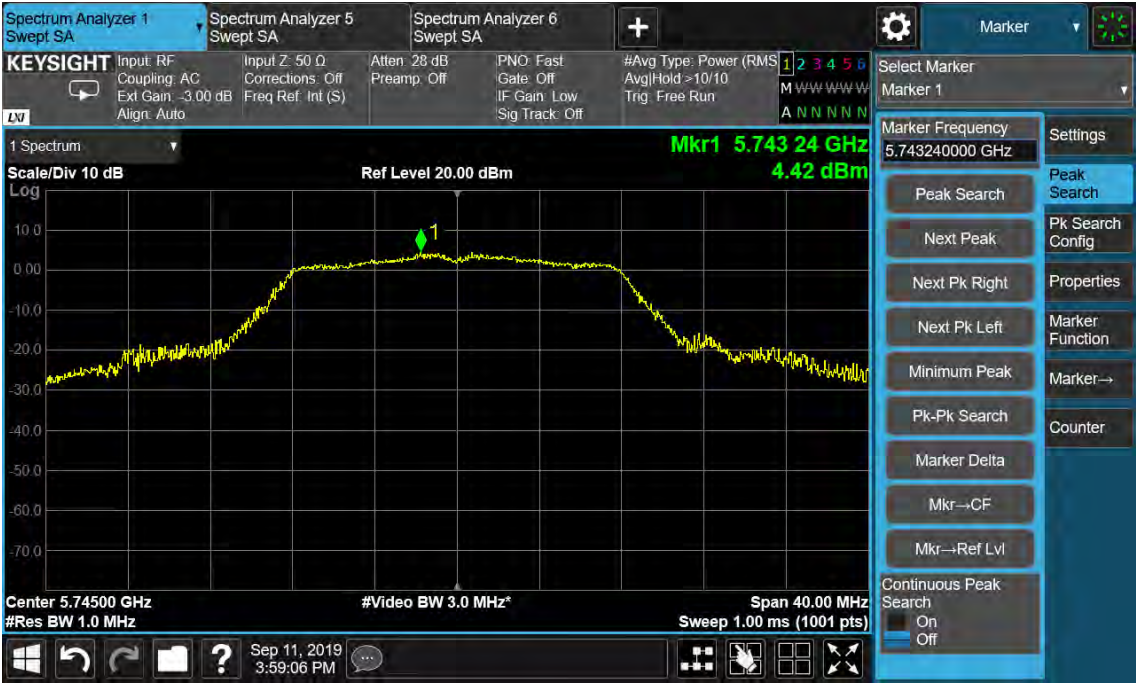
Figure 57: Power Spectral Density, 802.11a, 5745MHz
