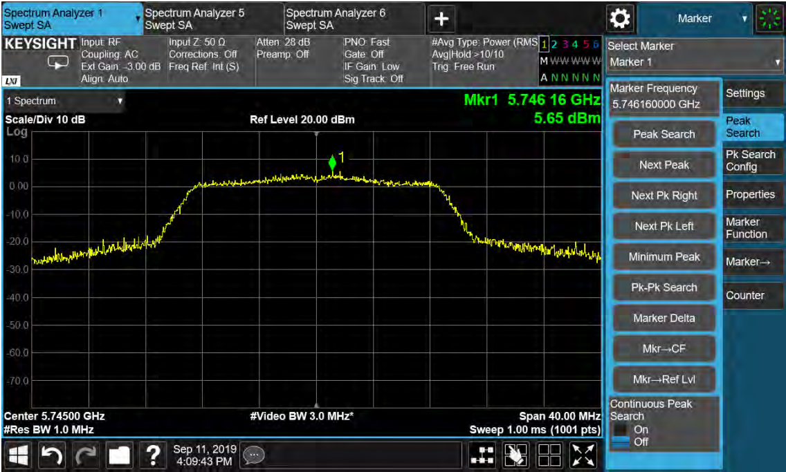
Figure 63: Power Spectral Density, 802.11ac(VHT20), 5745MHz
