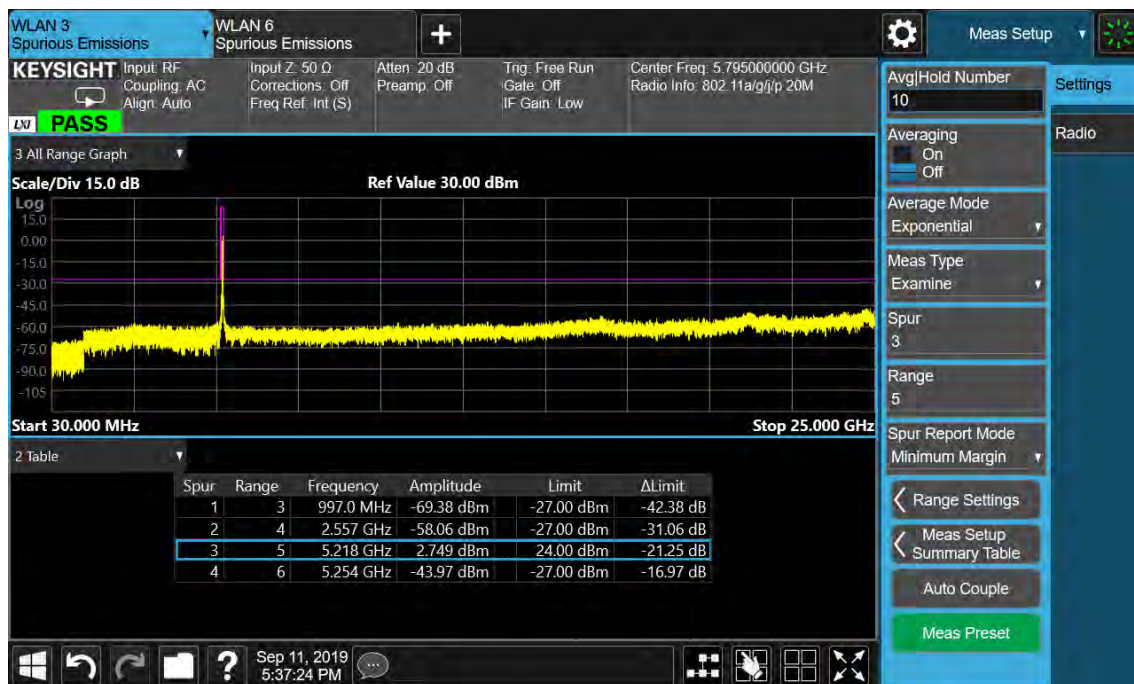
Figure 72: Undesirable Emission, 30MHz-25GHz, 802.11a, 5220MHz
