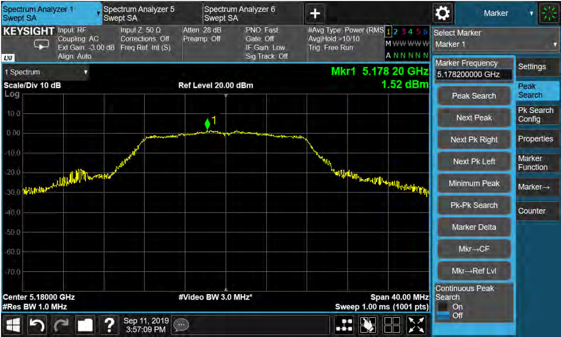
Figure 43: Power Spectral Density, 802.11a, 5180MHz
