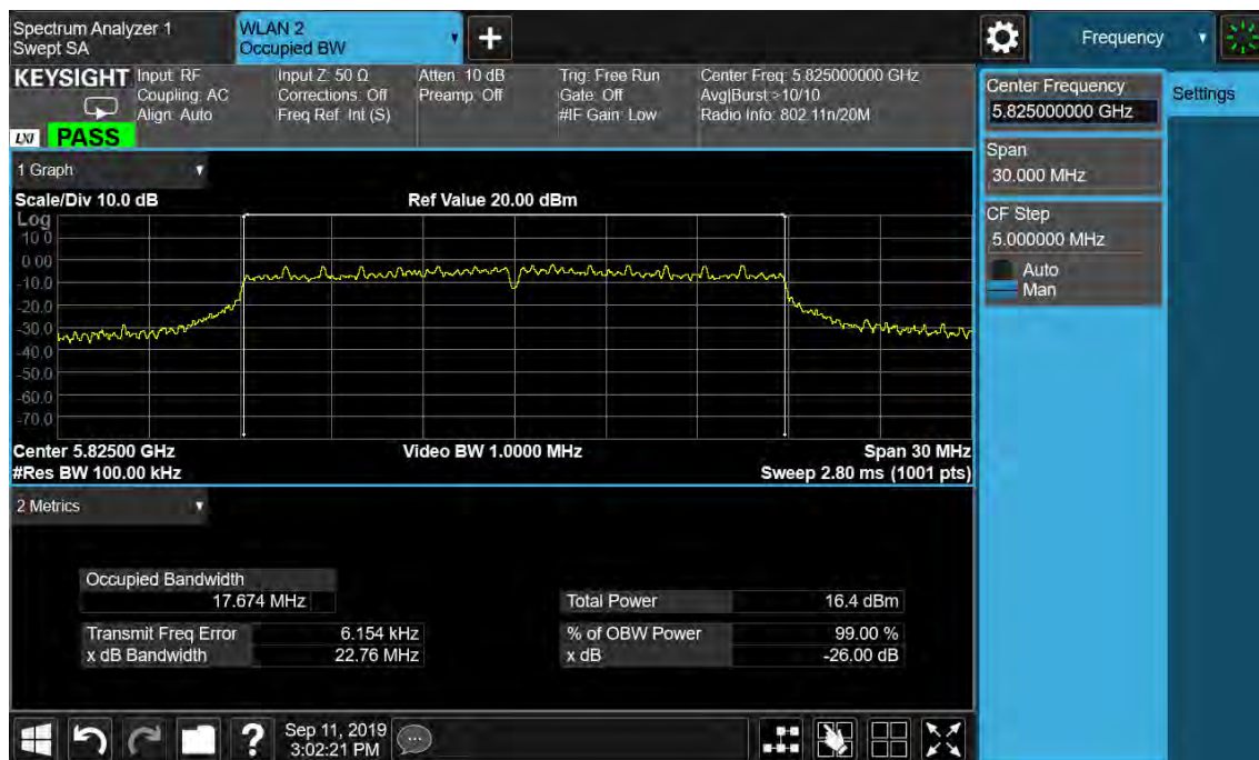
Figure 20: 26dB Bandwidth and 99% Bandwidth, 802.11n(HT20), 5825MHz
