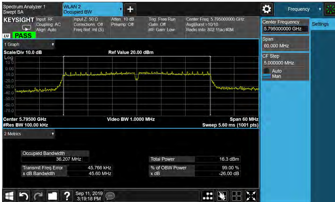
Figure 27: 26dB Bandwidth and 99% Bandwidth, 802.11ac(VHT40), 5785MHz
