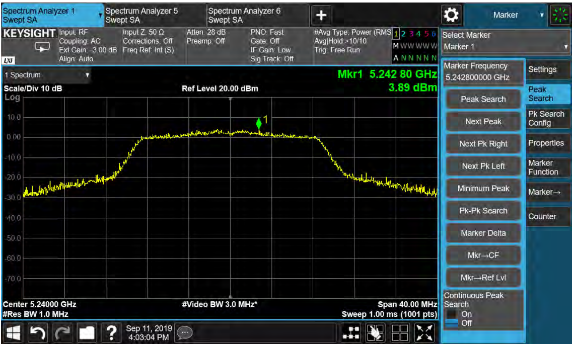
Figure 48: Power Spectral Density, 802.11n(HT20), 5240MHz
