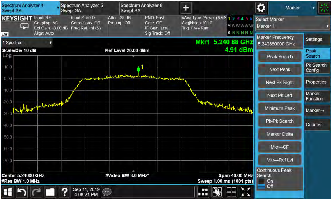
Figure 51: Power Spectral Density, 802.11ac(VHT20), 5240MHz
