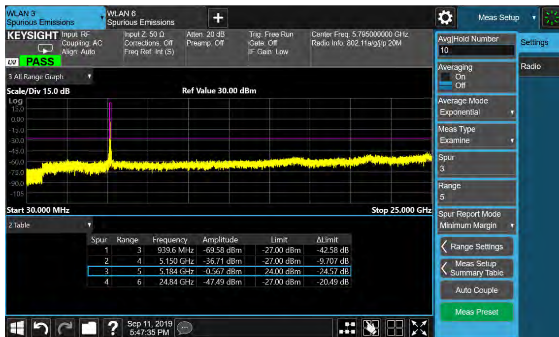
Figure 80: Undesirable Emission, 30MHz-25GHz, 802.11n(HT40), 5190MHz
