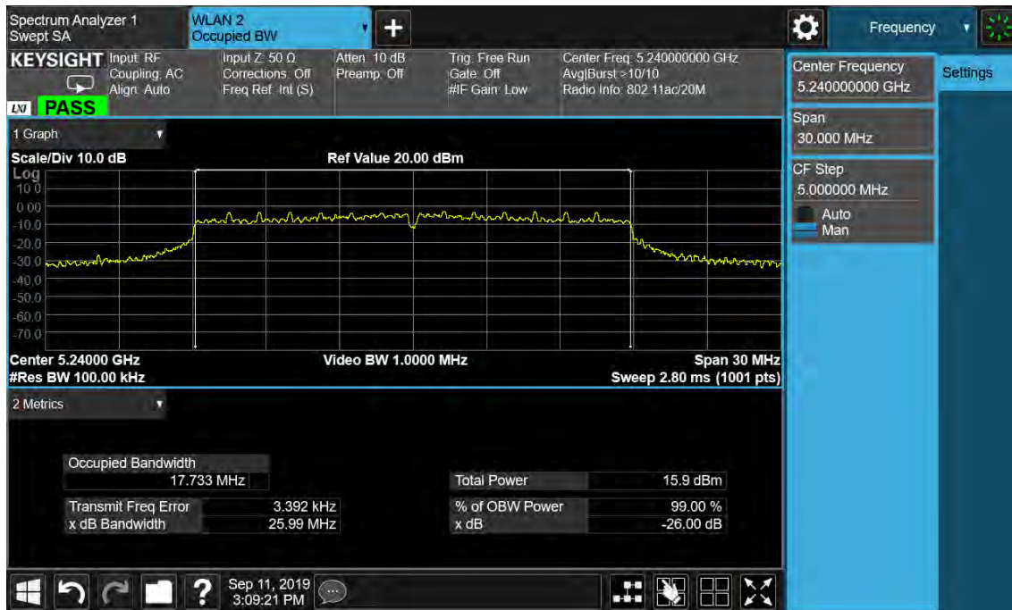
Figure 9: 26dB Bandwidth and 99% Bandwidth, 802.11ac(VHT20), 5240MHz
