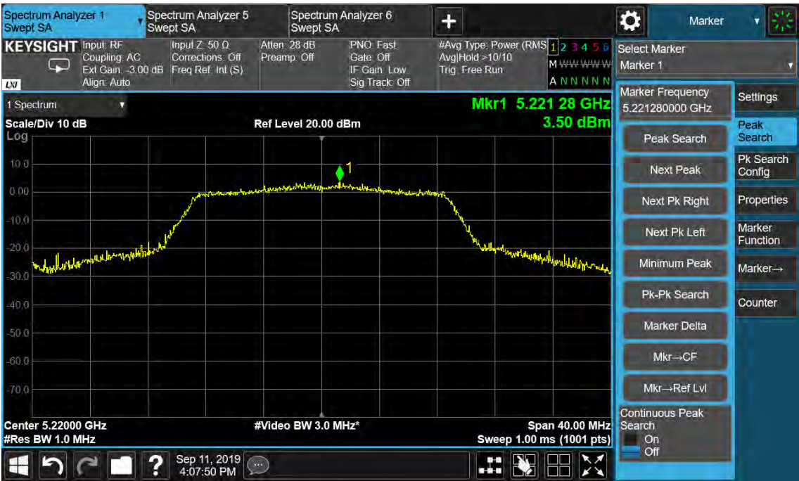
Figure 50: Power Spectral Density, 802.11ac(VHT20), 5220MHz
