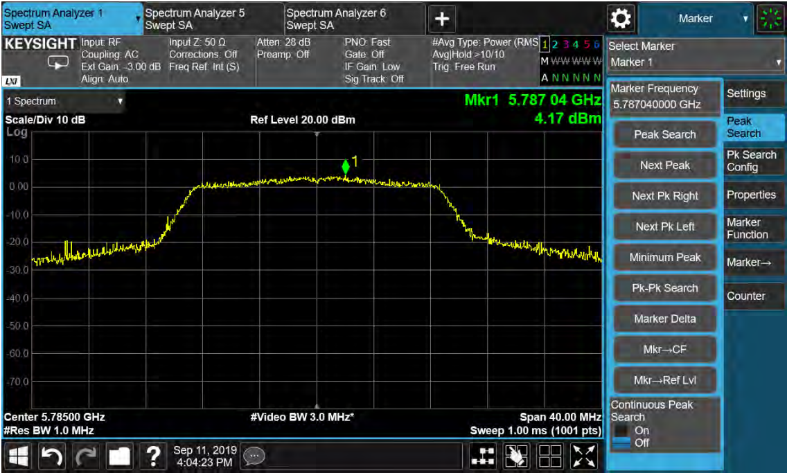
Figure 61: Power Spectral Density, 802.11n(HT20), 5785MHz
