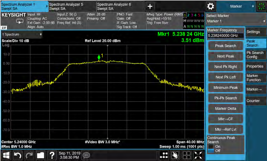
Figure 45: Power Spectral Density, 802.11a, 5240MHz
