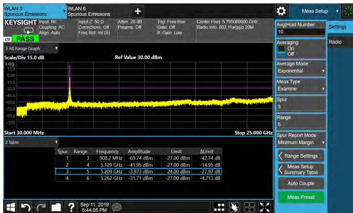
Figure 84: Undesirable Emission, 30MHz-25GHz, 802.11ac(VHT80), 5210MHz
