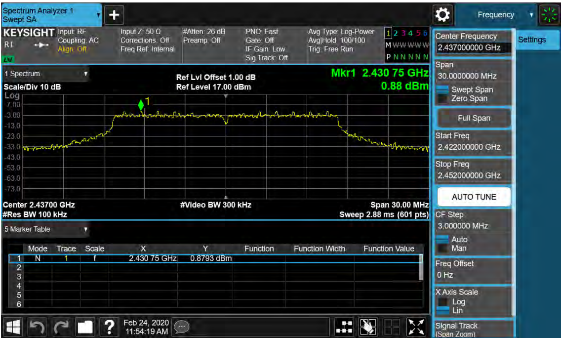
Figure 29: Conducted Spurious Emission & Authorized-band band-edge, 802.11g, 2437MHz Carrier Level
