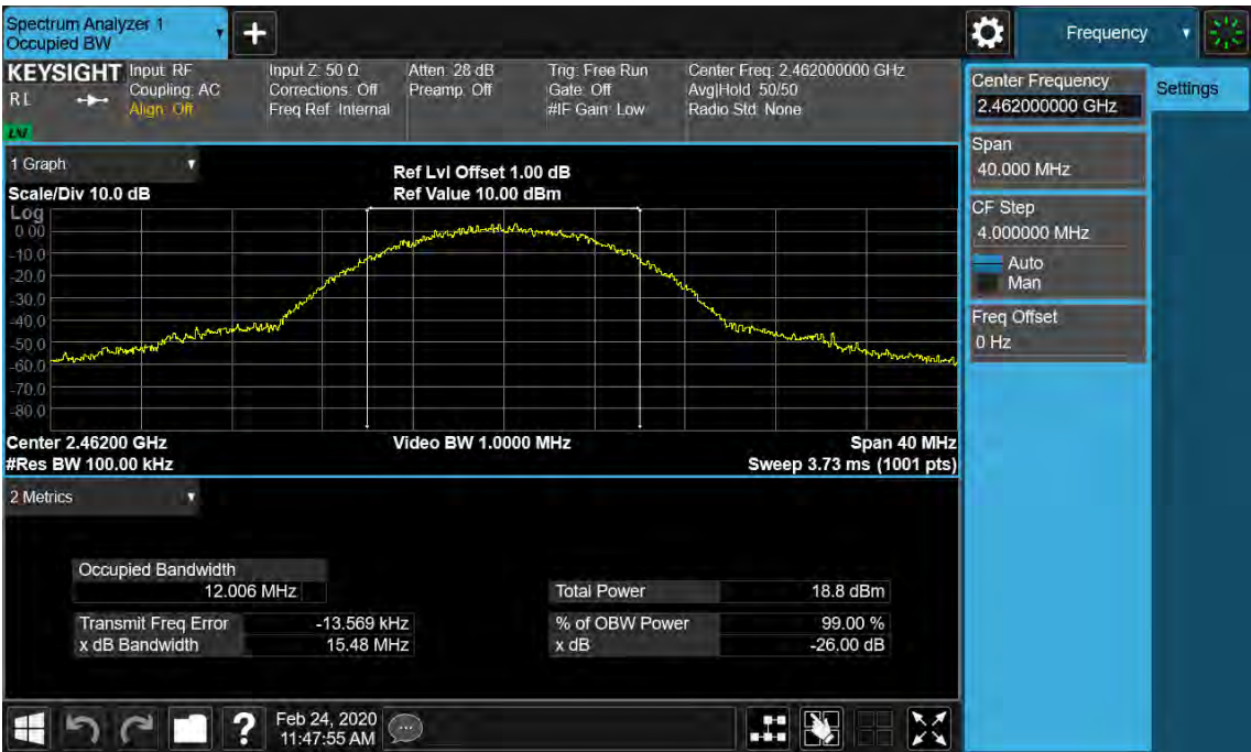
Figure 4: 6dB Bandwidth and 99% Bandwidth, 802.11g, 2412MHz
