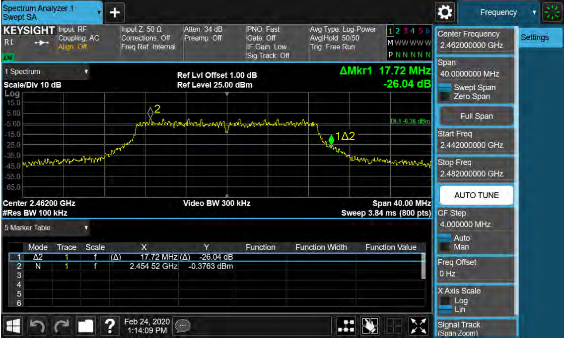
Figure 9: 6dB Bandwidth and 99% Bandwidth, 802.11n(HT20), 2462MHz
