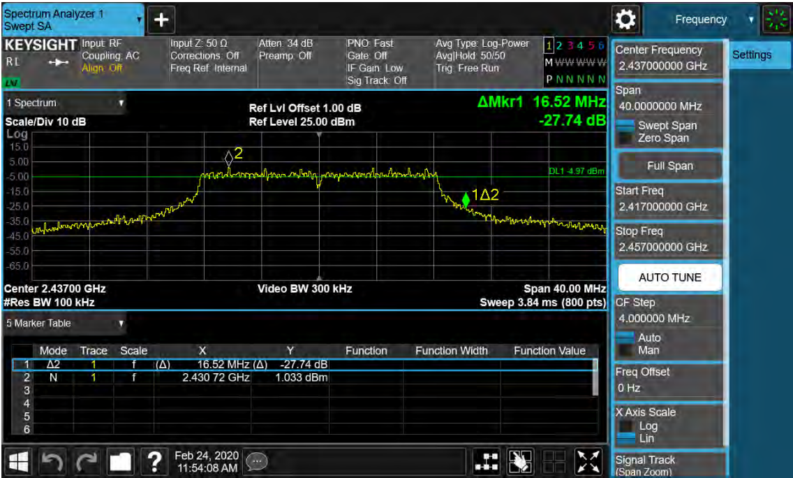
Figure 7: 6dB Bandwidth and 99% Bandwidth, 802.11n(HT20), 2412MHz
