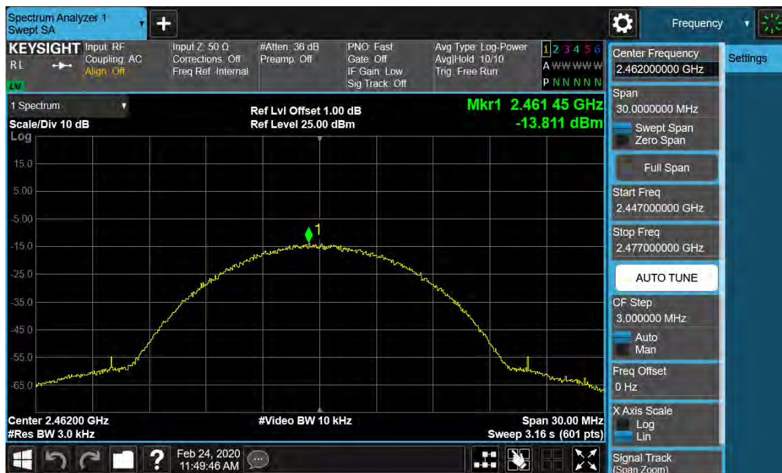
Figure 15: Power Spectral Density, 802.11b, 2462MHz
