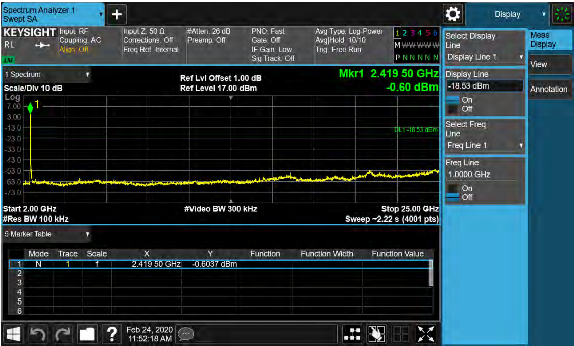
Figure 29: Conducted Spurious Emission & Authorized-band band-edge, 802.11g, 2437MHz Carrier Level
