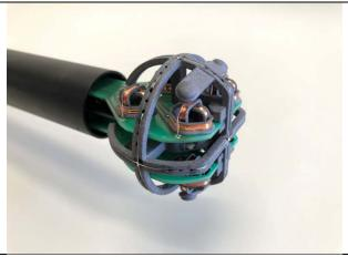
Test probe, without the casing
