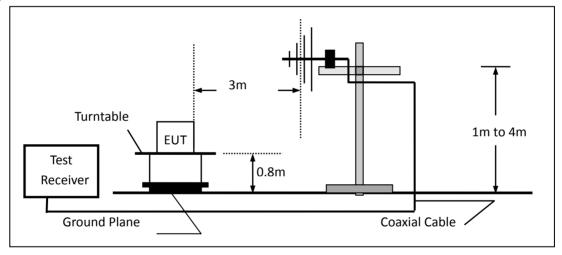
(c) For radiated emissions above 1000MHz
