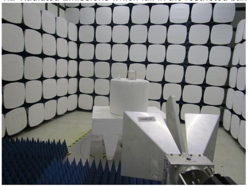
1.3 Radiated Spurious Emissions Test Setup
