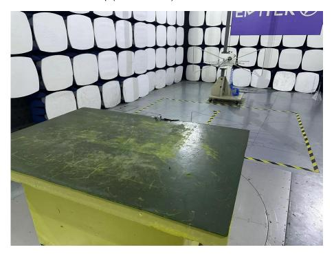
Spurious Emission Test Setup (Above 1GHz)
