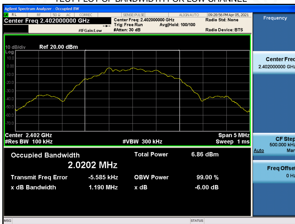
TEST PLOT OF BANDWIDTH FOR LOW CHANNEL
