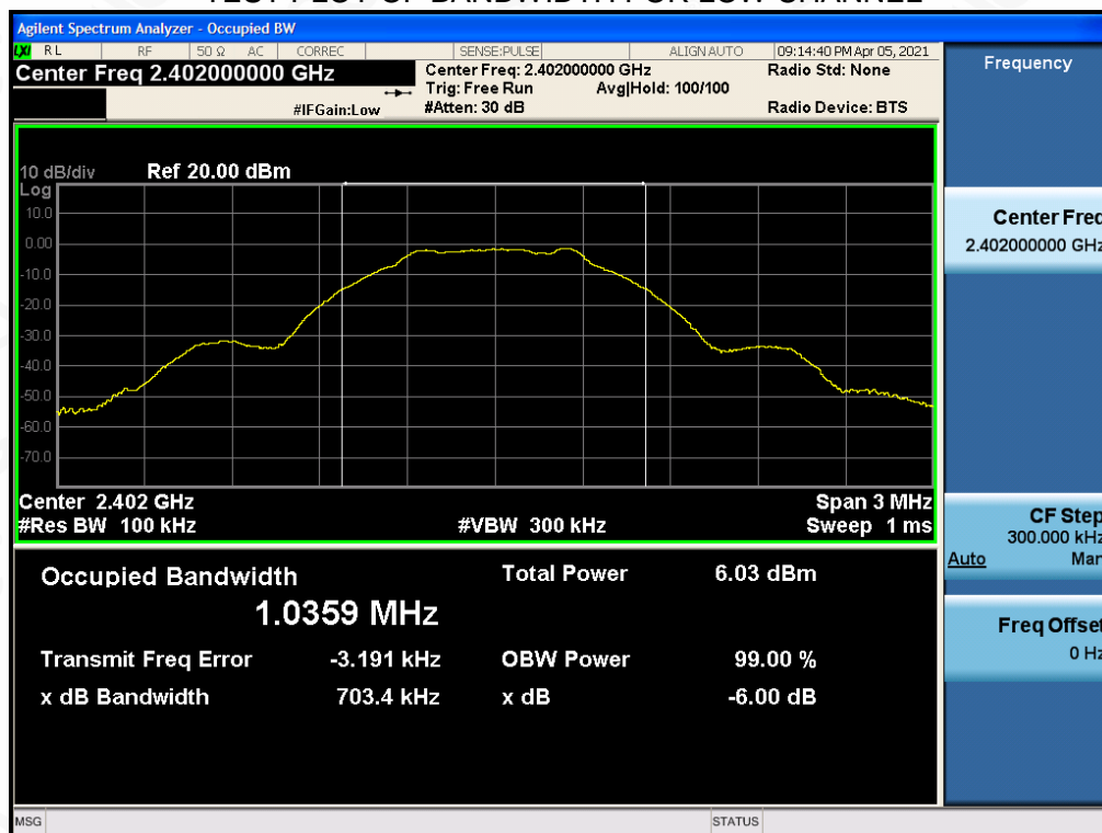
TEST PLOT OF BANDWIDTH FOR LOW CHANNEL
