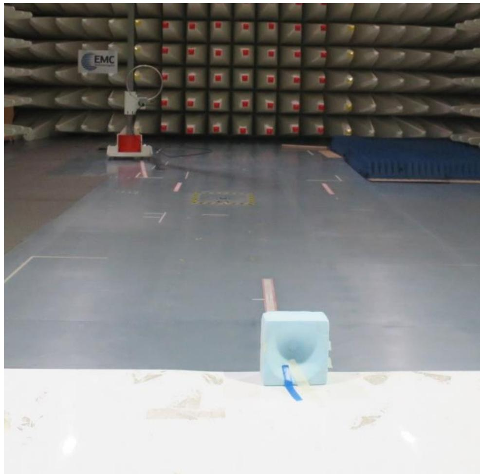
Radiated Emissions - 30 MHz to 1000 MHz
