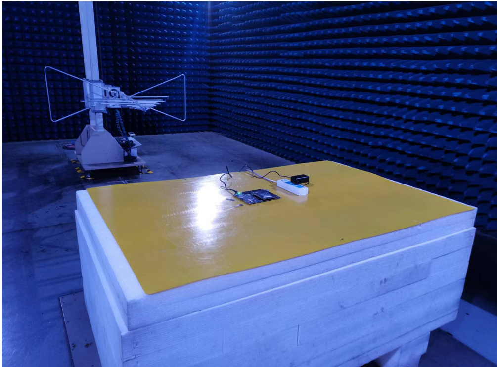
Photo of Radiated Emission Measurement (Above 1G)
