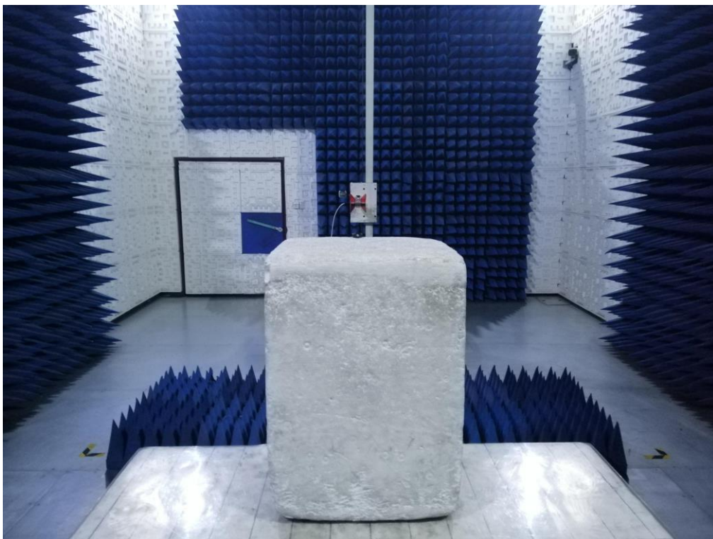
RADIATED EMISSION TEST SETUP ABOVE 1GHz
