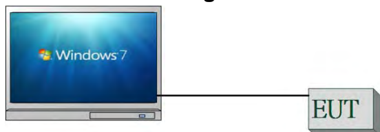
Fig. 2-1 Conducted (Antenna Port) Emission Configuration
