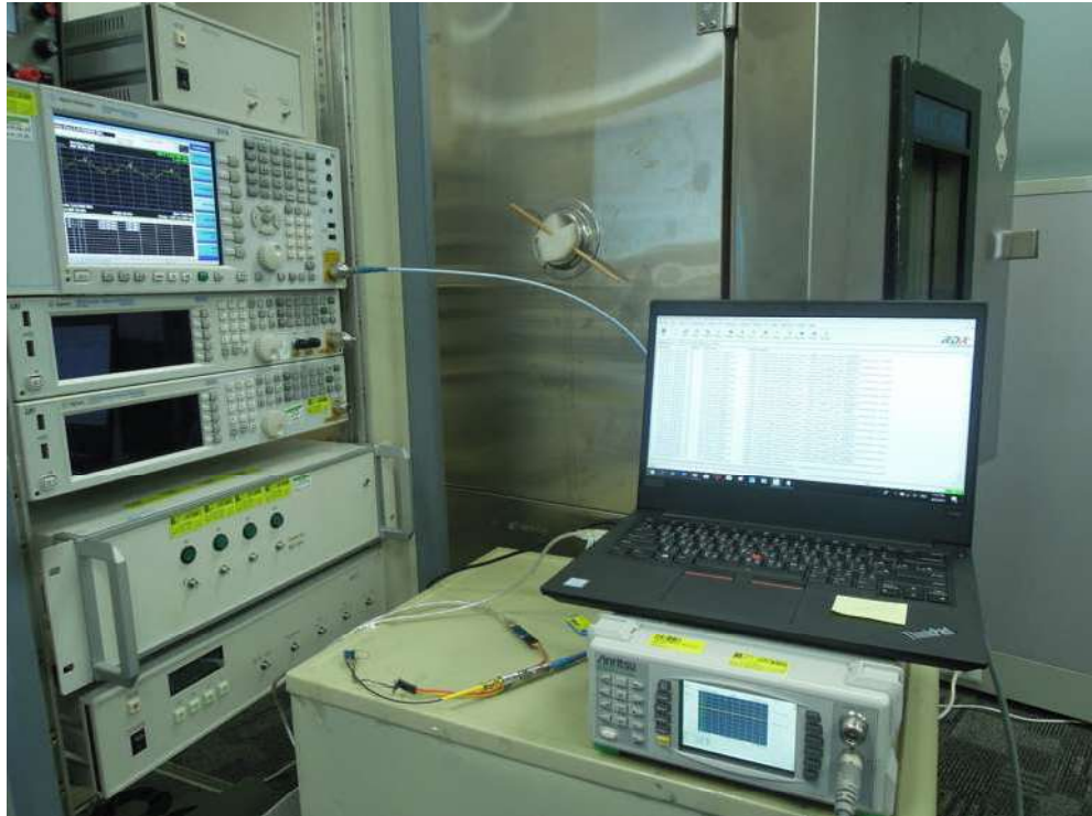
Photograph 5: Set-up for Conducted testing (View 1)
