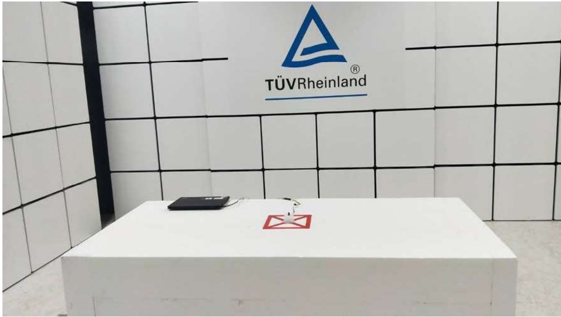
Photograph 1: Set-up for Spurious Emissions (Front View)
