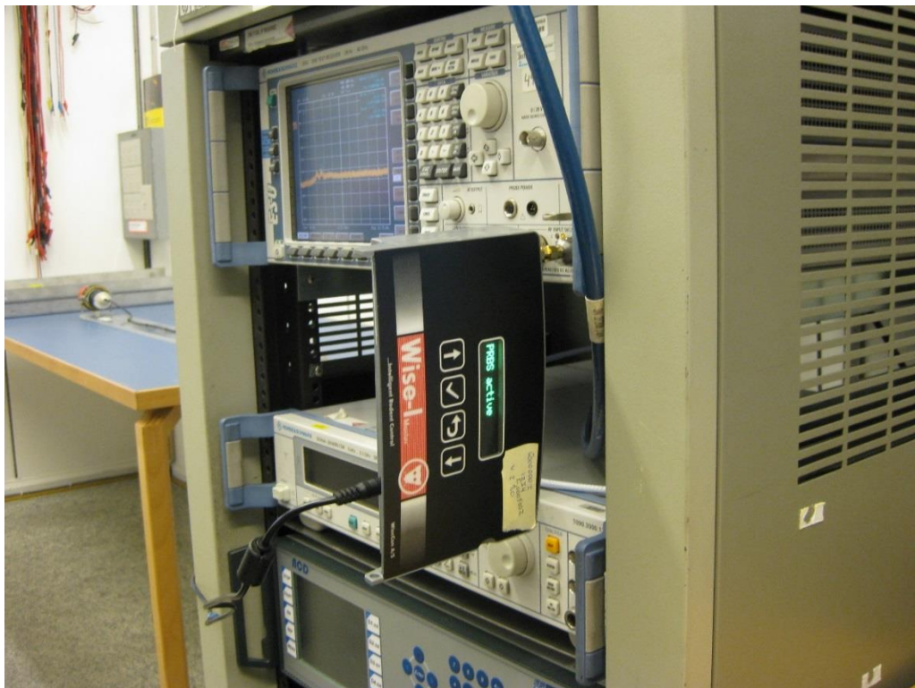
Photo 4.5.1 Test setup regarding measurement of conducted spurious emissions.
