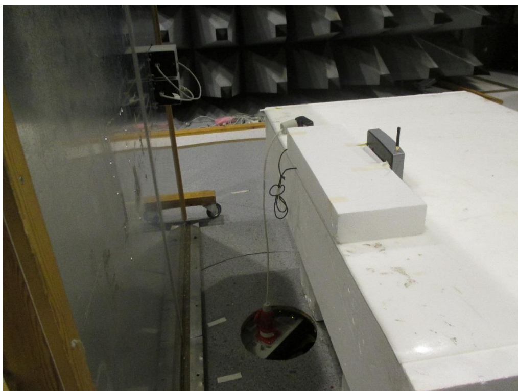
Photo 4.6.2 Test setup regarding measurement of radio frequency voltage on mains.
