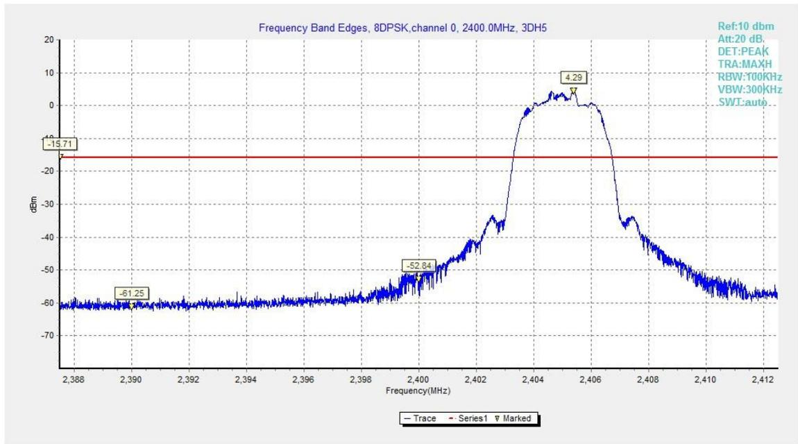
Fig.9. Frequency Band Edges: 8DPSK, Channel 0, Hopping Off
