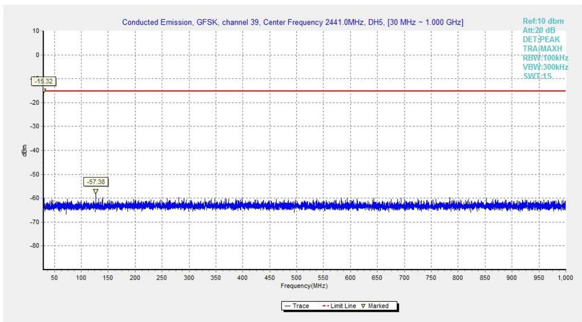
Fig.19. Conducted spurious emission: GFSK, Channel 39, 30MHz - 1GHz
