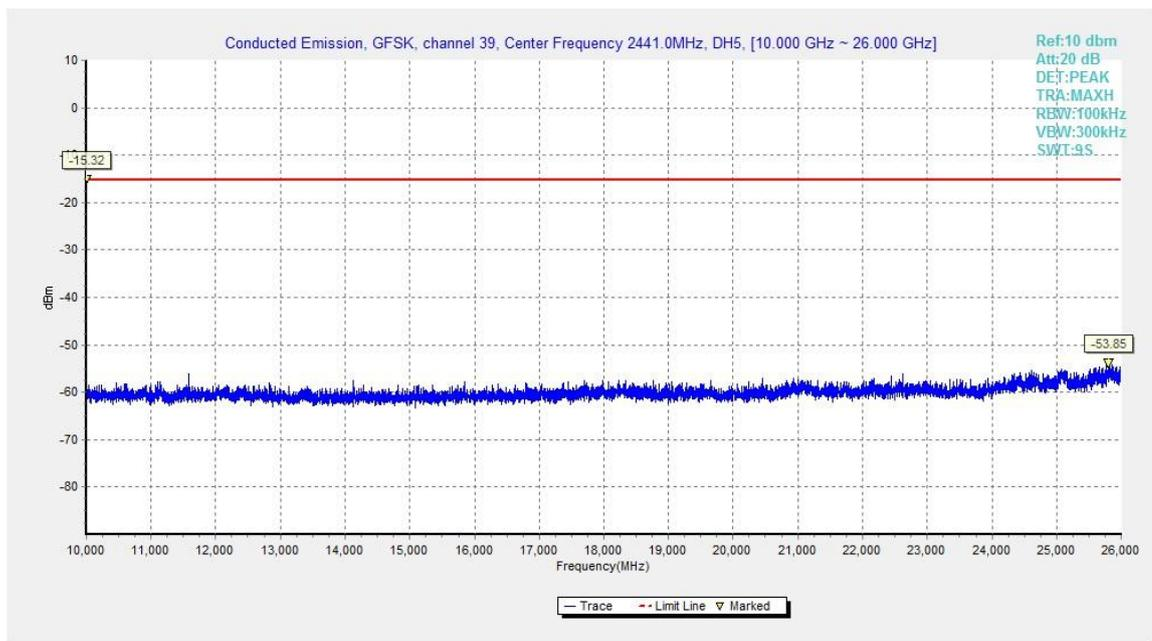
Fig.22. Conducted spurious emission: GFSK, Channel 39, 10GHz – 26GHz
