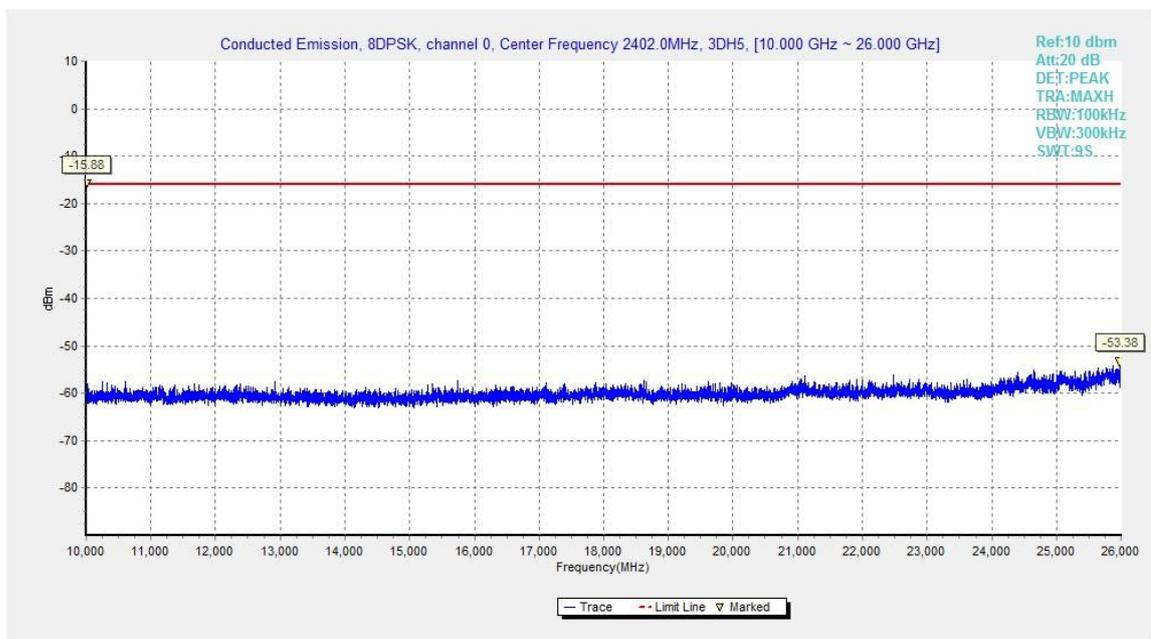
Fig.47. Conducted spurious emission: 8DPSK, Channel 0,10GHz - 26GHz
