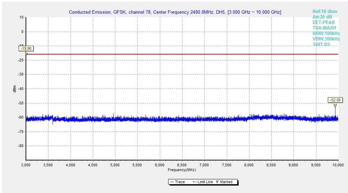
Fig.26. Conducted spurious emission: GFSK, Channel 78, 3GHz - 10GHz
