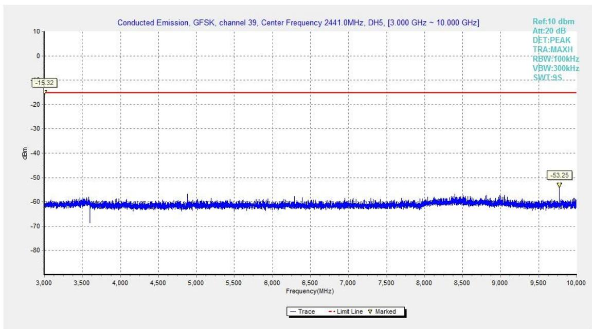
Fig.21. Conducted spurious emission: GFSK, Channel 39, 3GHz – 10GHz
