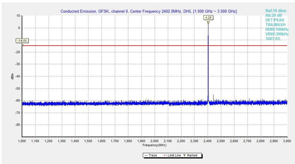
Fig.15. Conducted spurious emission: GFSK, Channel 0, 1GHz - 3GHz
