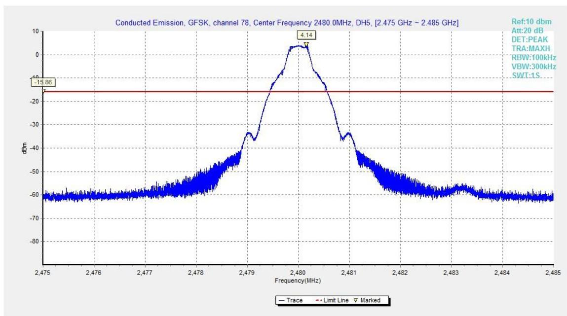
Fig.23. Conducted spurious emission: GFSK, Channel 78, 2480MHz
