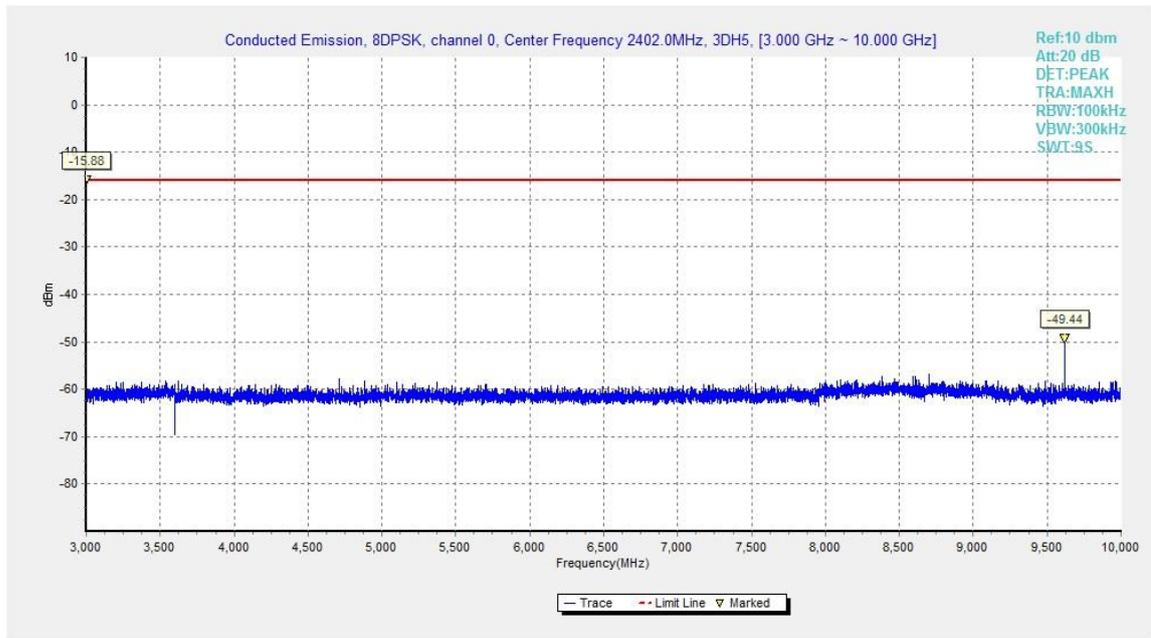
Fig.46. Conducted spurious emission: 8DPSK, Channel 0, 3GHz - 10GHz
