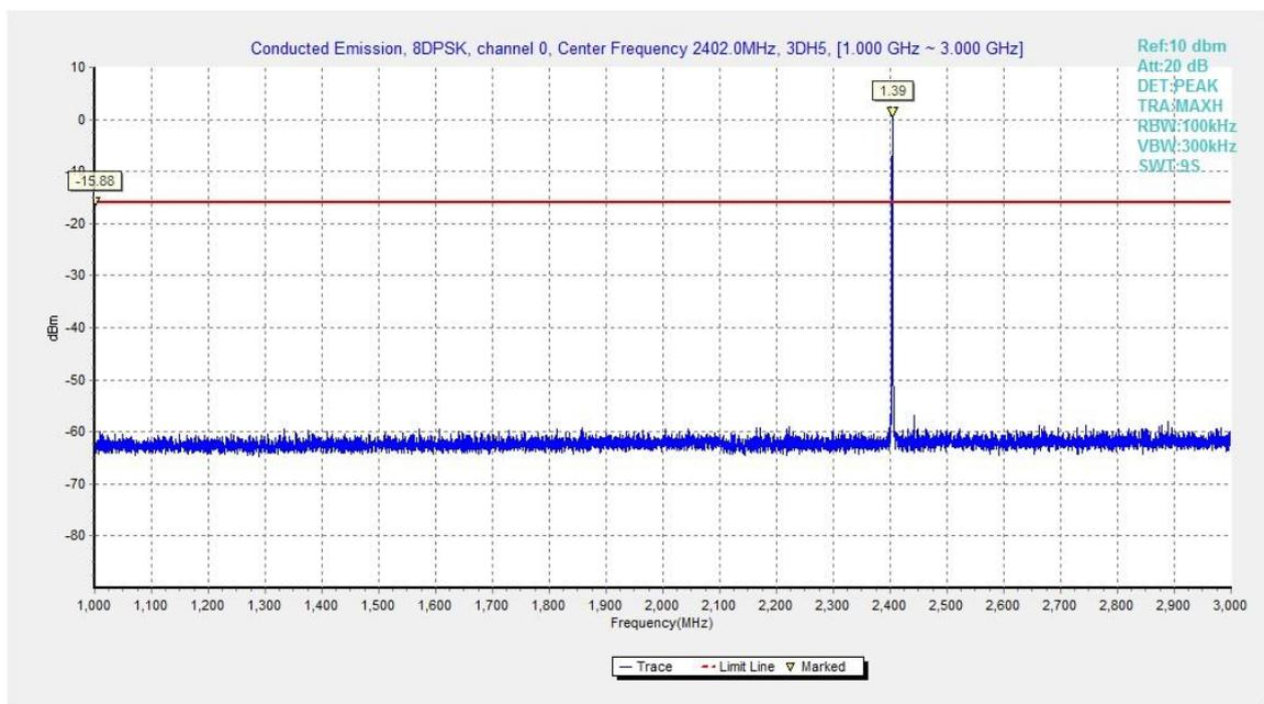
Fig.45. Conducted spurious emission: 8DPSK, Channel 0, 1GHz - 3GHz
