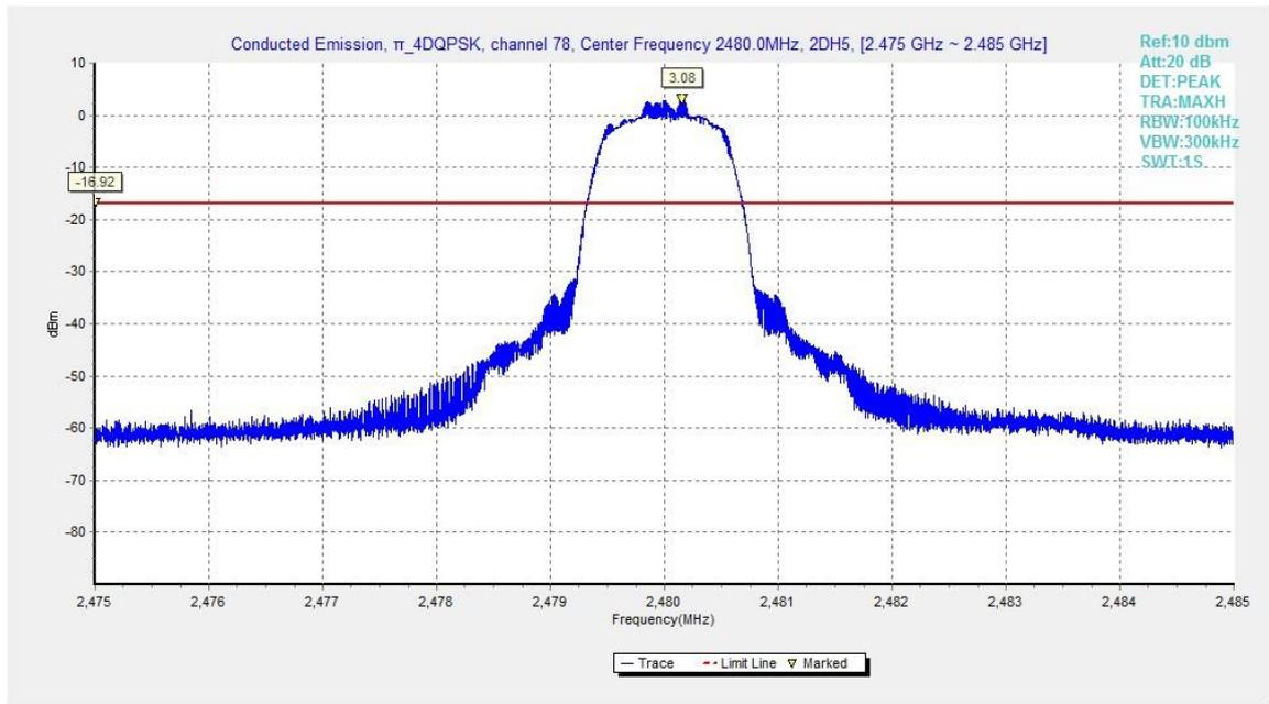
Fig.38. Conducted spurious emission:  $\pi/4$  DQPSK, Channel 78, 2480MHz
