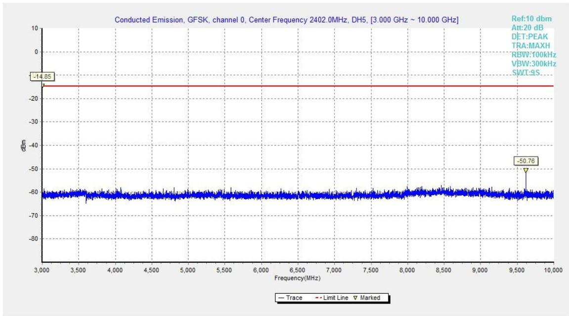
Fig.16. Conducted spurious emission: GFSK, Channel 0, 3GHz - 10GHz
