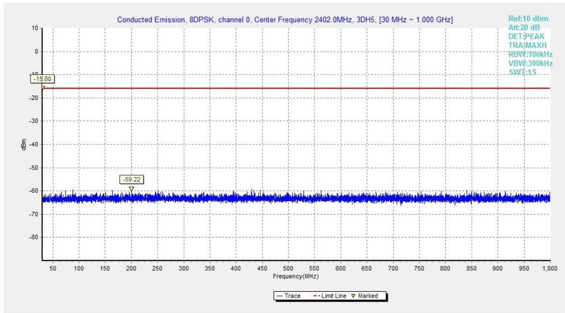
Fig.44. Conducted spurious emission: 8DPSK, Channel 0, 30MHz - 1GHz
