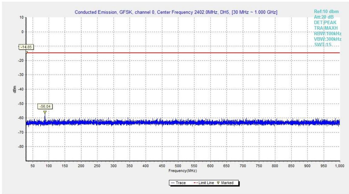
Fig.14. Conducted spurious emission: GFSK, Channel 0, 30MHz - 1GHz
