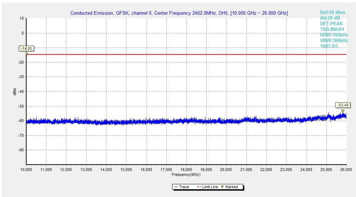
Fig.17. Conducted spurious emission: GFSK, Channel 0, 10GHz - 26GHz
