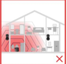
The positioning of the Hub might initially be limited, because it needs to connect to an ethernet port that connects back to your modem or home router. If you can move the Hub into a more centralized location, it will improve the performance of the entire system.
