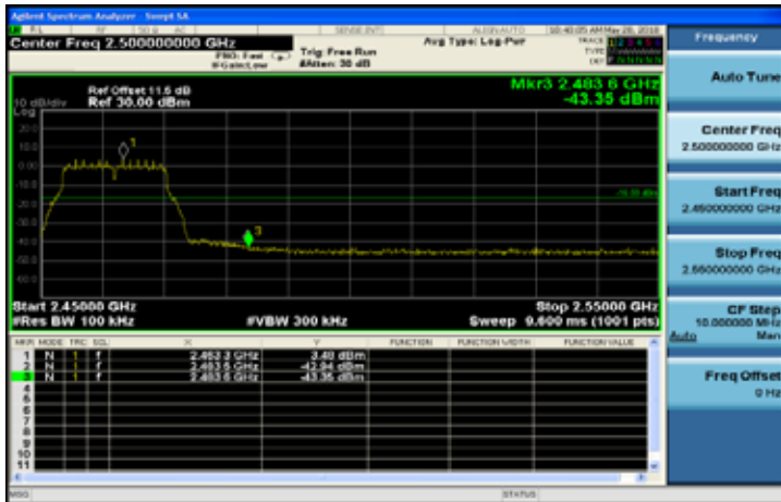
802.11g: Band Edges Test Data CH-High
