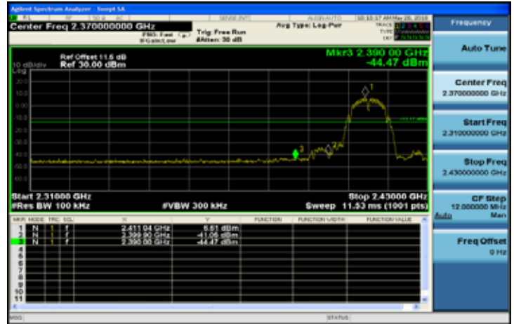
802.11b: Band Edges Test Data CH-High
