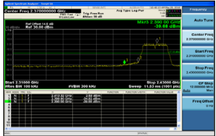
802.11n_HT20: Band Edges Test Data CH-High
