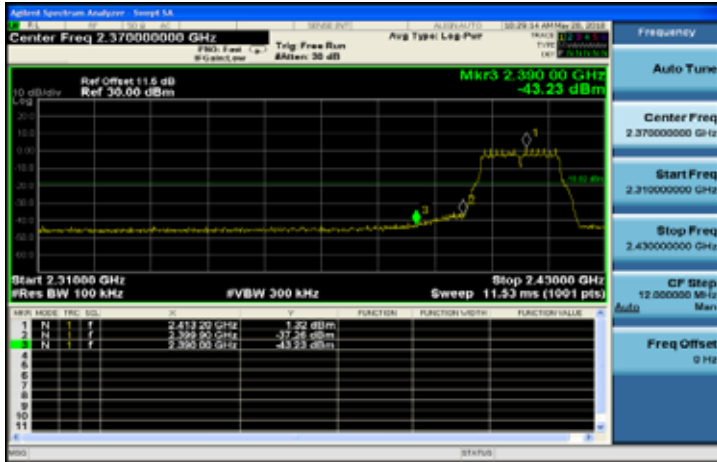
802.11g: Band Edges Test Data CH-High
