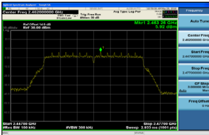
802.11n_HT20 Reference Level of Emission Limit(CH-High)
