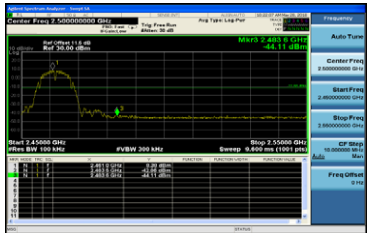
802.11b: Band Edges Test Data CH-High
