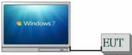
Fig. 2-2 Conducted (Antenna Port) Emission Configuration
