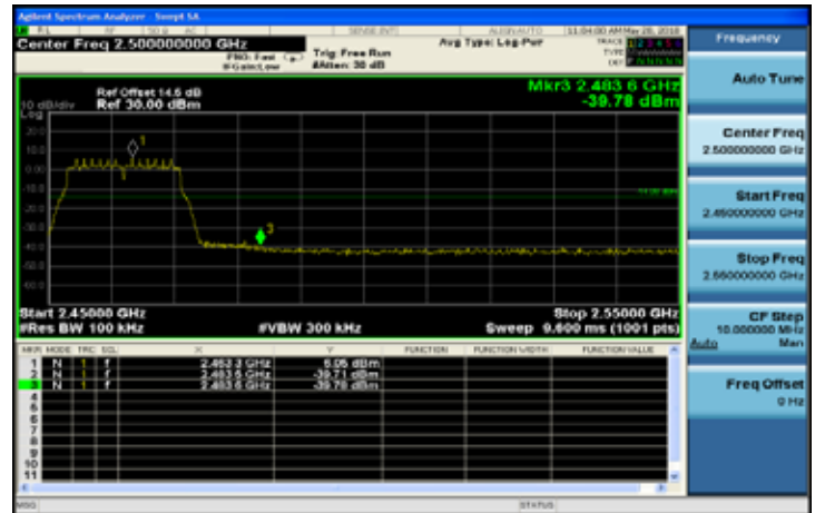
802.11n_HT20: Band Edges Test Data CH-High
