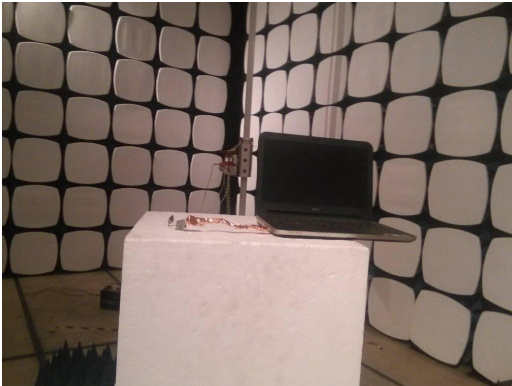
RADIATED EMISSION TEST SETUP ABOVE 1GHZ
