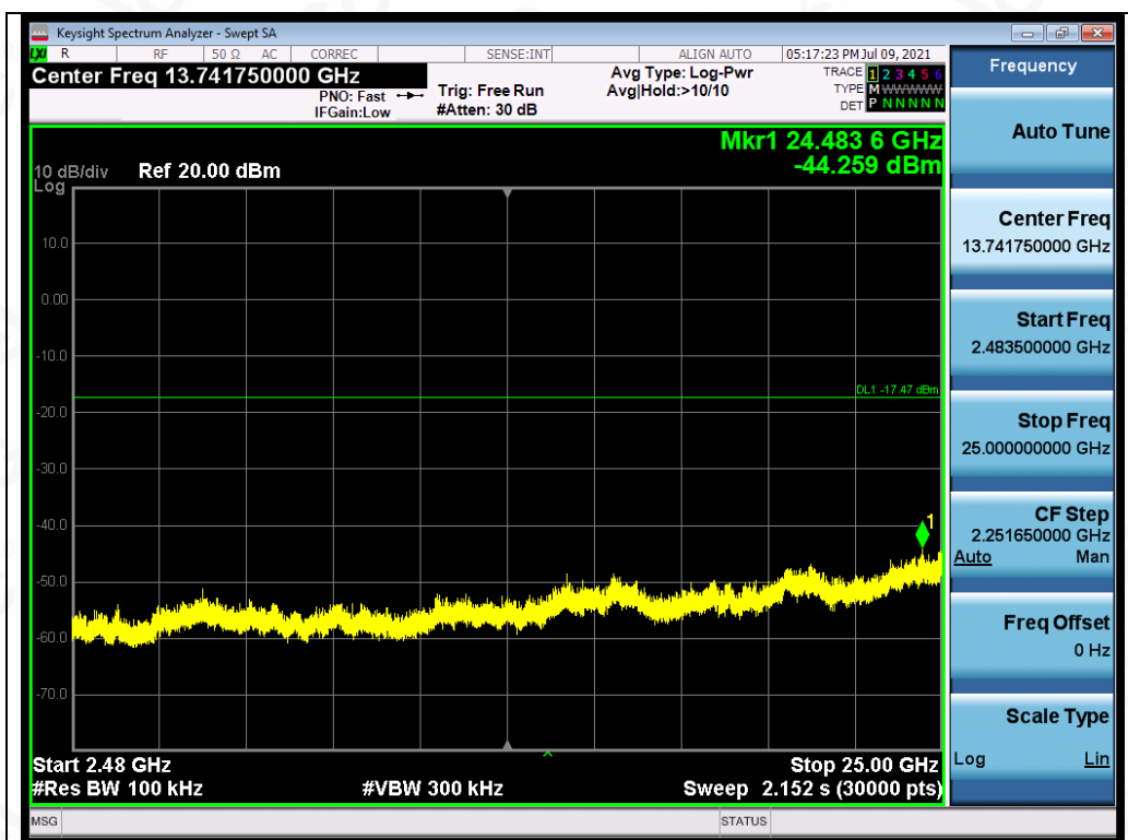
Test_Graph_EDR_ANT1_2402_3Mbps_Higher Band Emissions
