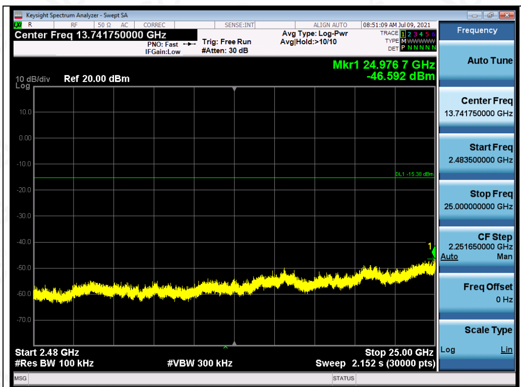
Test_Graph_BR_ANT1_2402_1Mbps_Higher Band Emissions
