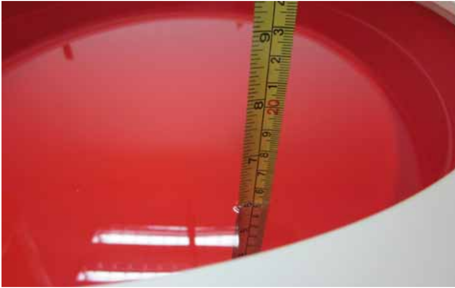
Figure 4.4: Liquid depth in the Flat Phantom
